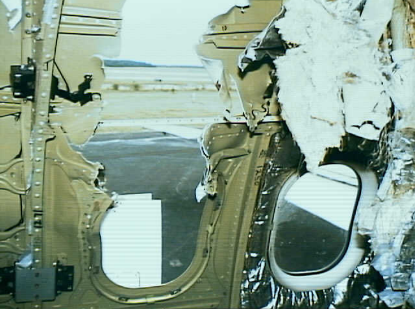
Photo 9. Interior view of left fuselage penetration damage adjacent to row 37.
