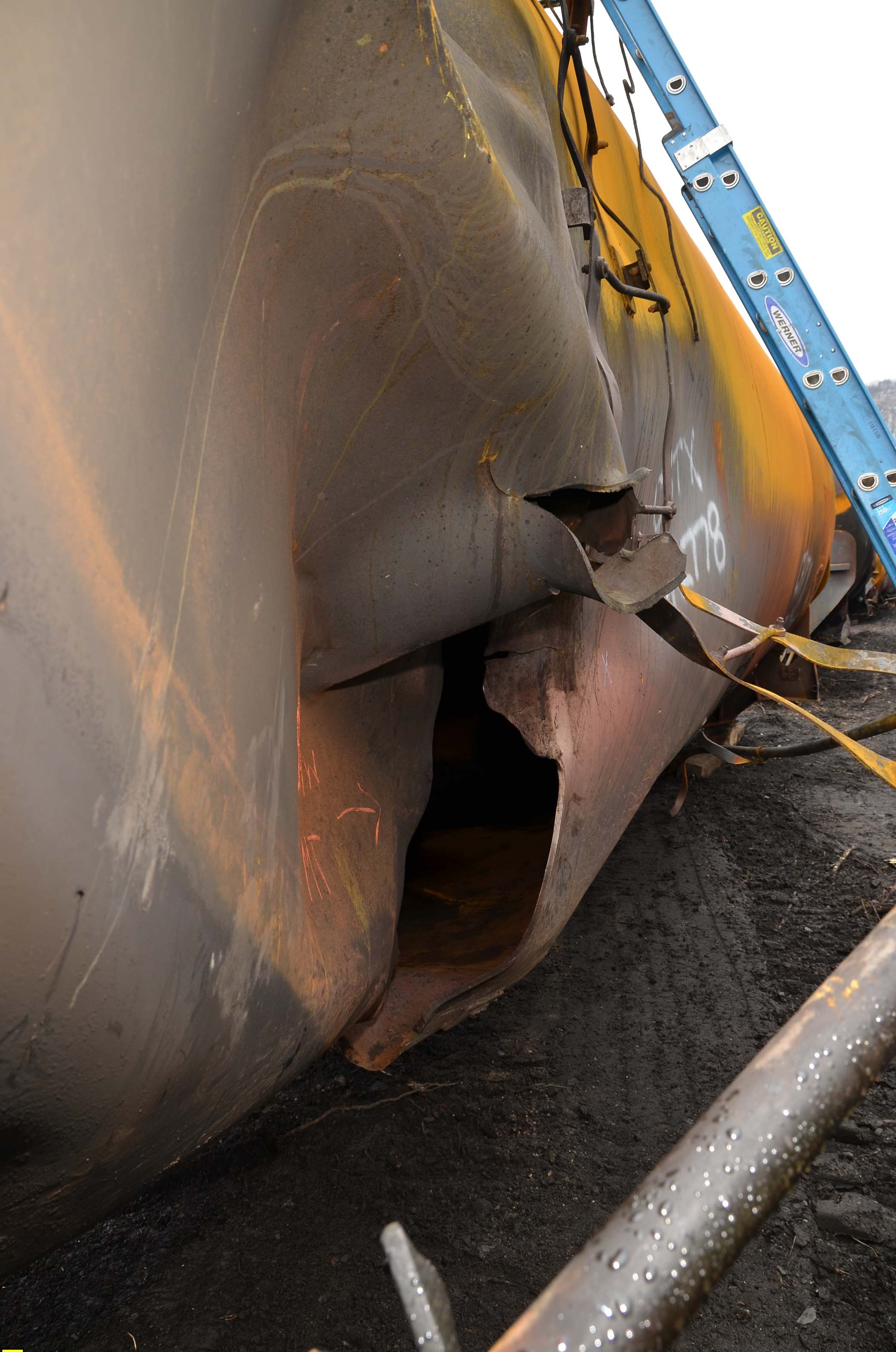
Photo 9 - Tank Car CBTX742778, Position 19, Puncture, March 3, 2015
