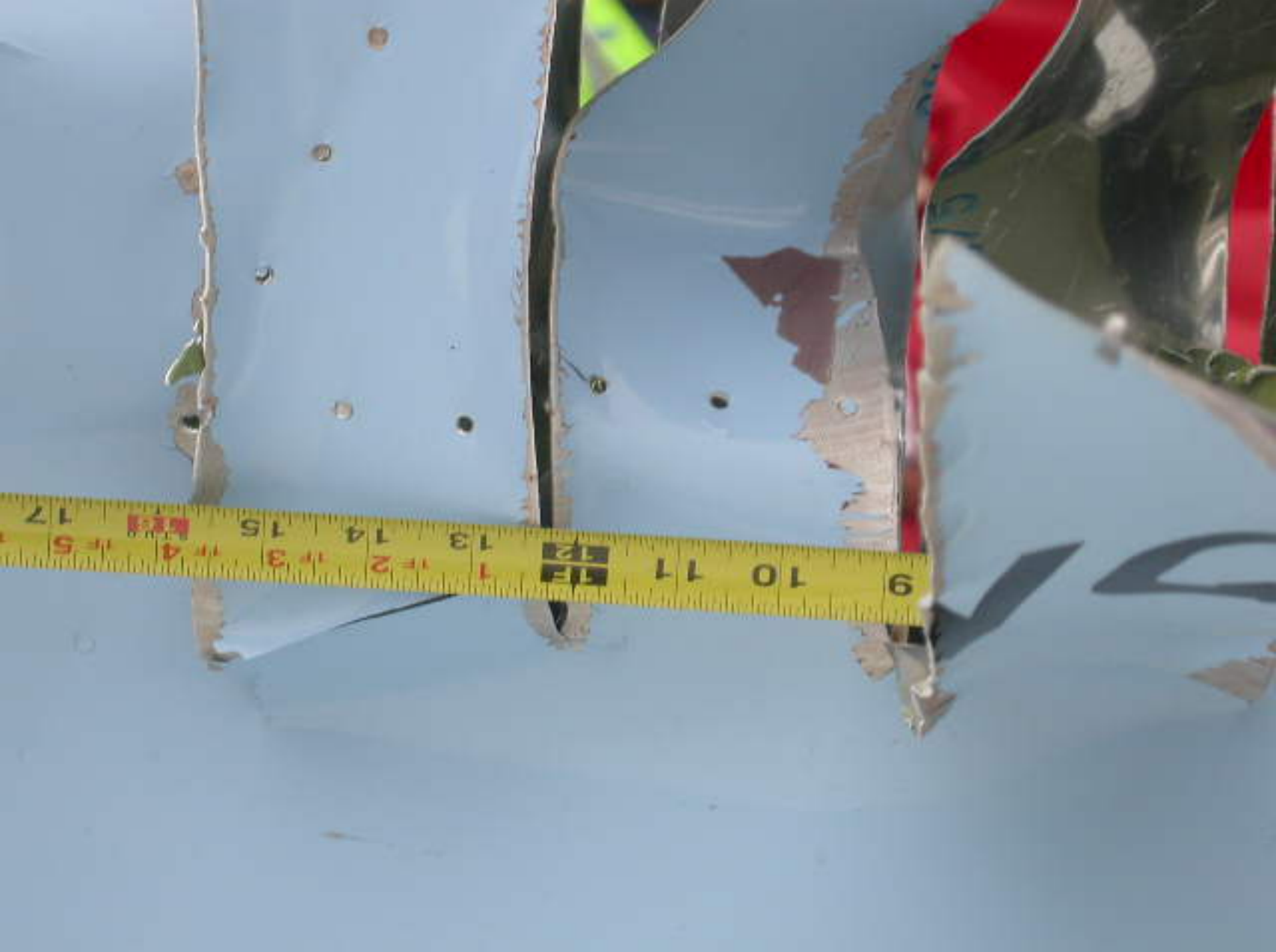
Photo 8. Measurement of Propeller Slashes on Fuselage
