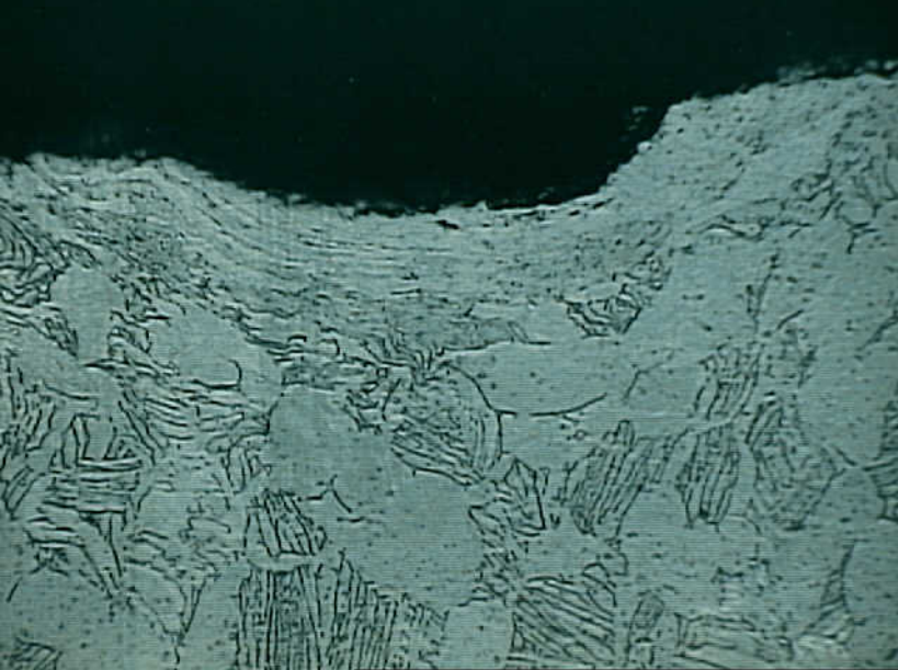
Photo 8. Longitudinal section of hole 2 through a BEA indication, arrow A in photo 7. The microstructure showing plastic deformation to a depth of up to 35um (1.38 mills) created by a impression of a chip. Mag.
