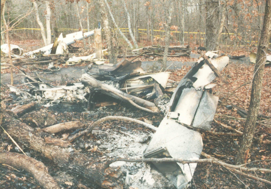
Photo 8. Left Wing, Inboard Section, Trailing Edge & Left Wing Flap
