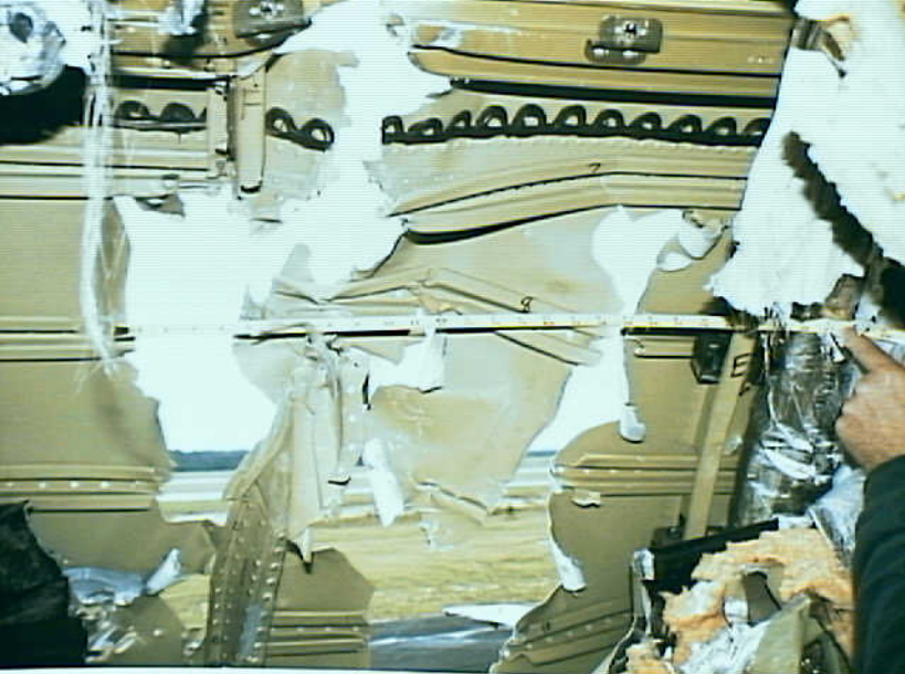
Photo 8. Interior view of left fuselage penetration damage adjacent to row 37.
