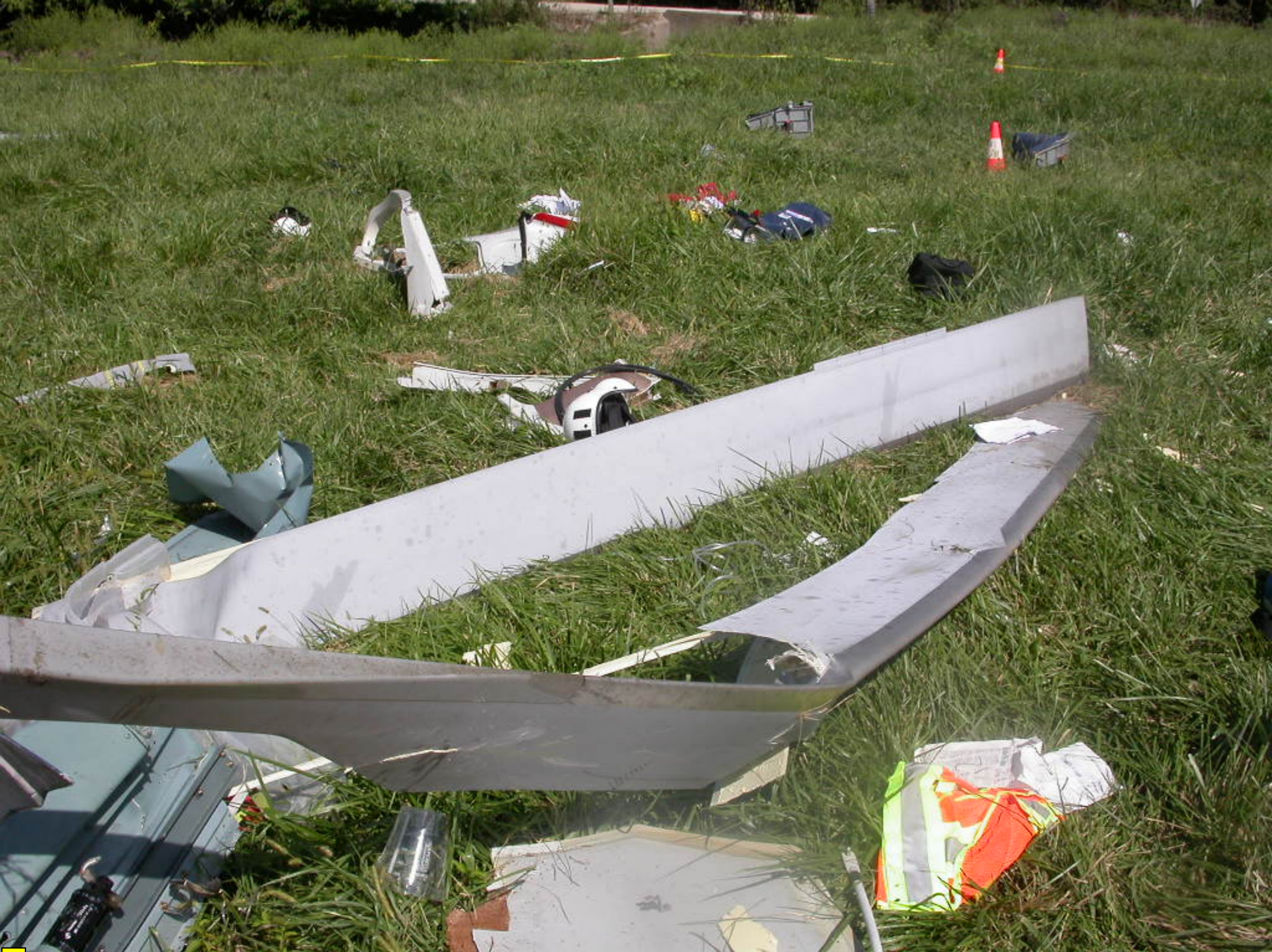
Photo 8: View of two main rotor blades
