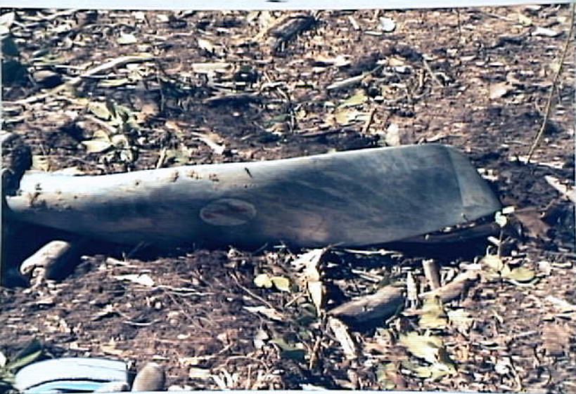
Photo 8: View of other propeller blade. Note spanwise and chordwise scratches.
