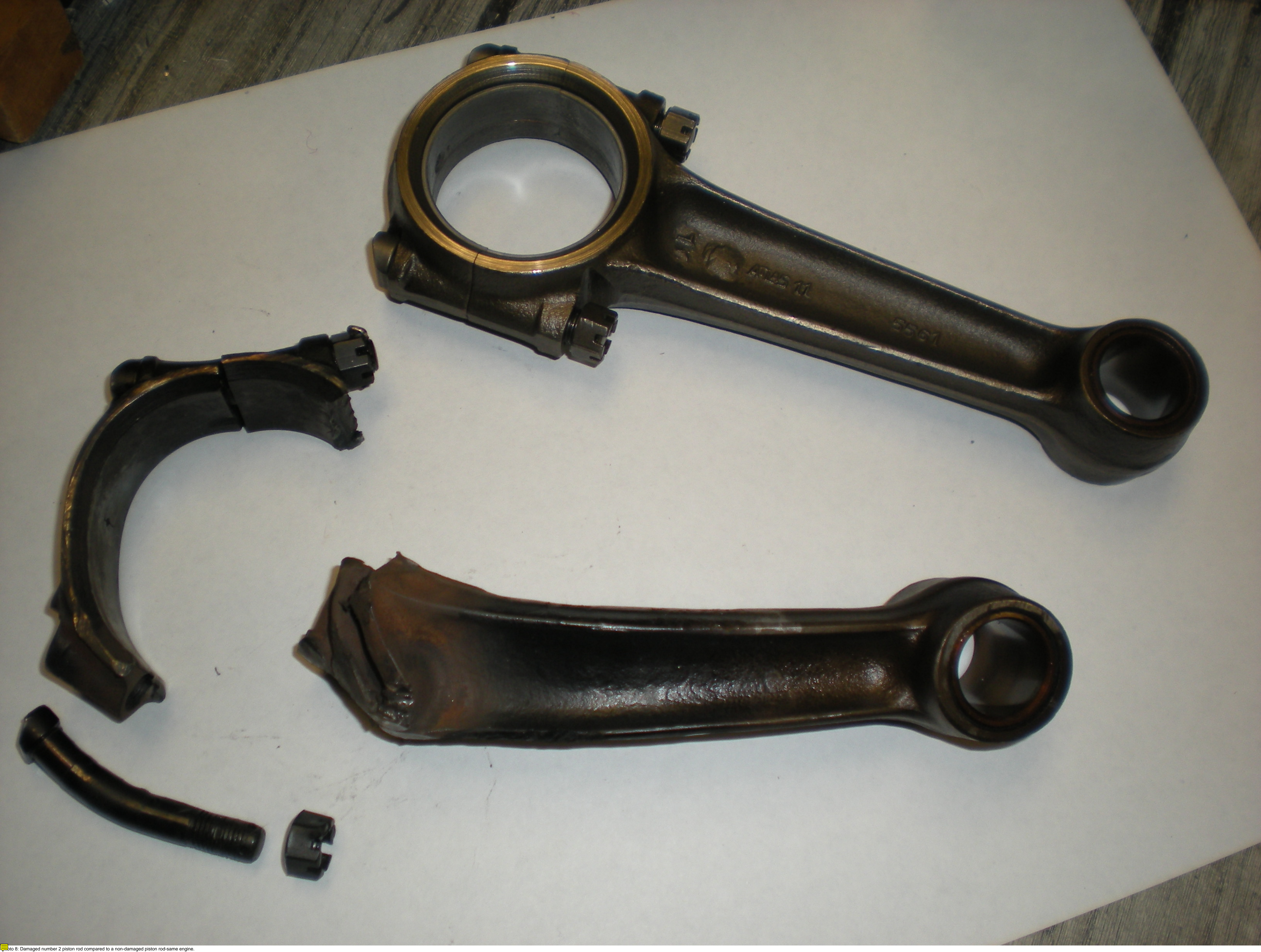
Photo 8: Damaged number 2 piston rod compared to a non-damaged piston rod-same engine.
