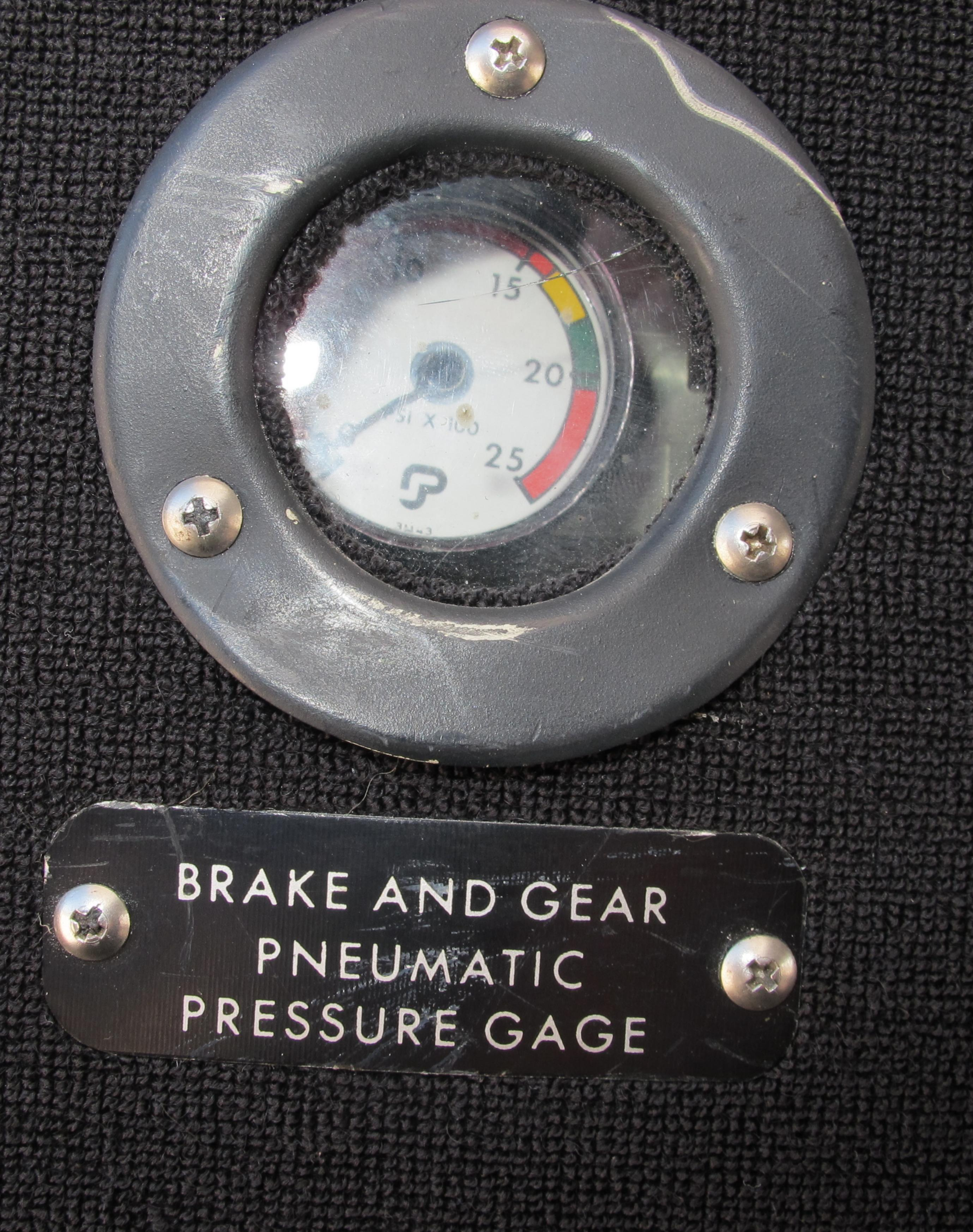
to 8: Brake and Gear Pneumatic Pressure Gage
