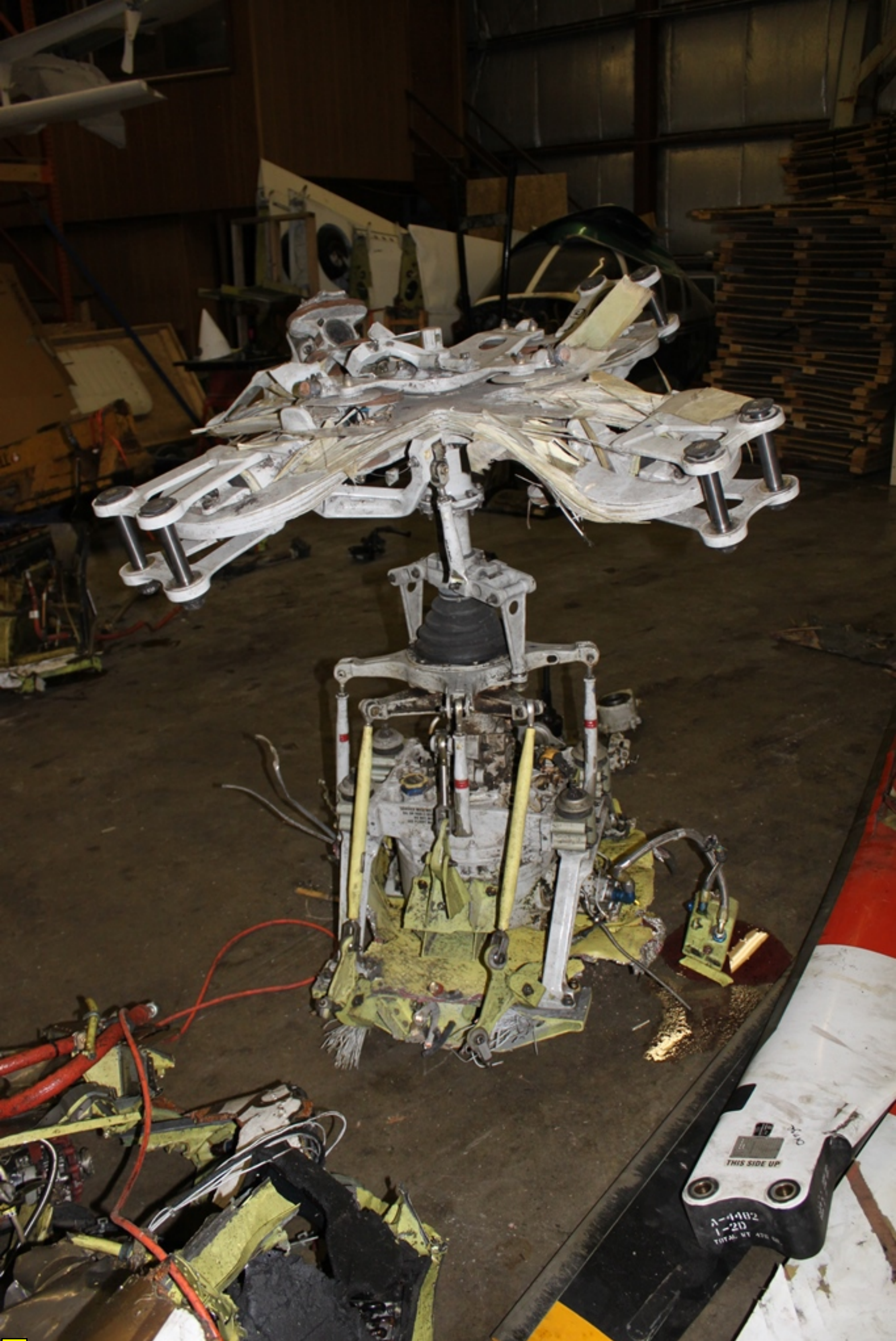
Photo 7. Main Rotor Hub/Transmission (Blades Removed)
