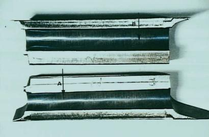
Photo 7. Hole #2 drilled with standard cutting data with HSS. The arrows show BEA indications consisting of impressions of chips smeared on the hole surface.
