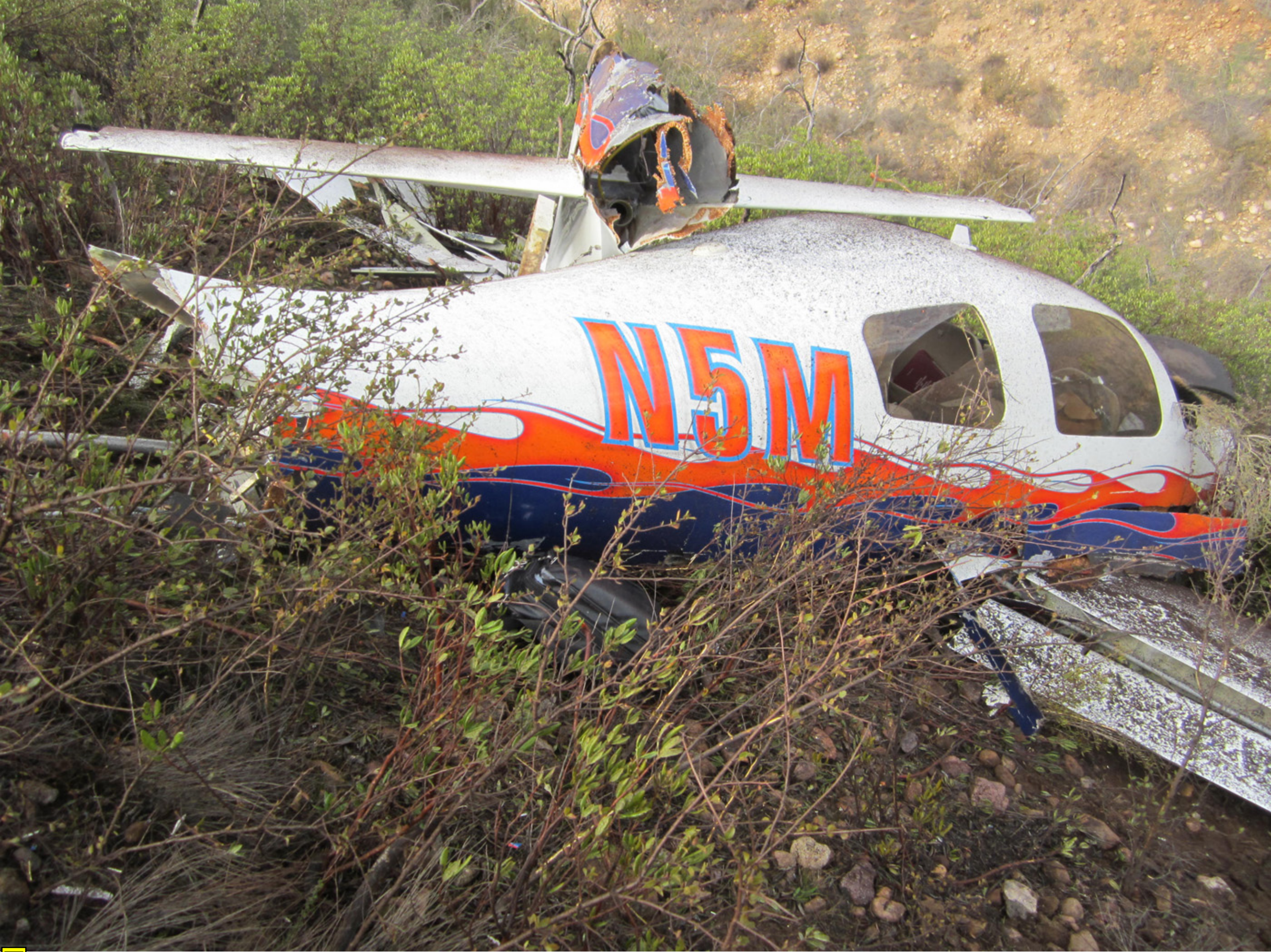
Photo 7 - View of broken empennage
