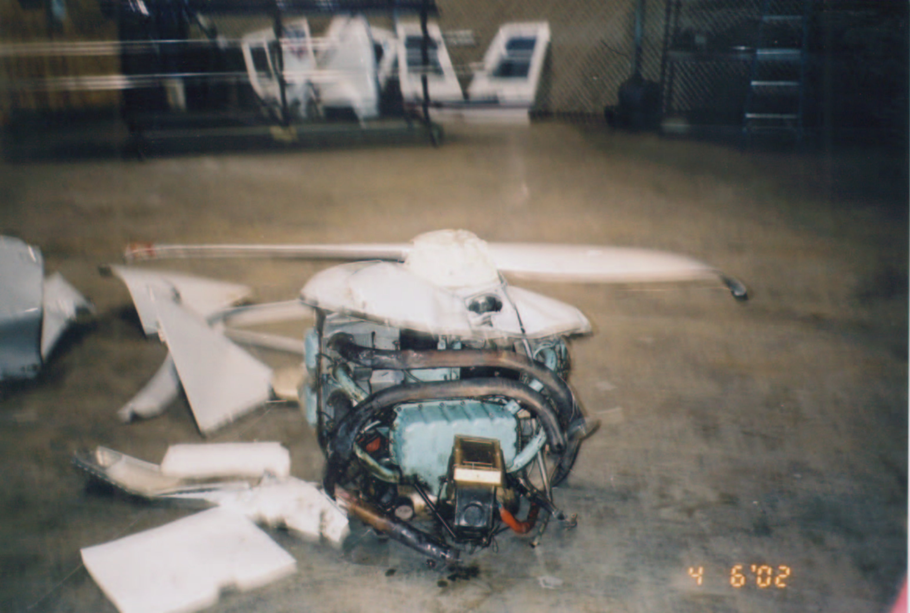
Photo 7 - View of N5293H separated engine assembly
