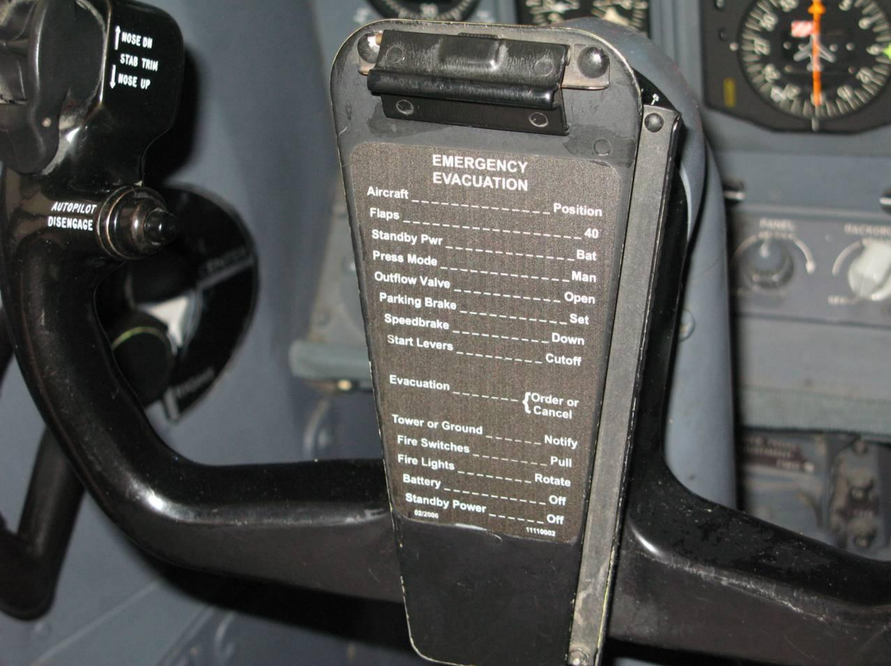
Photo 7 - Cockpit Control Yoke Showing Checklist for Emergency Evacuation
