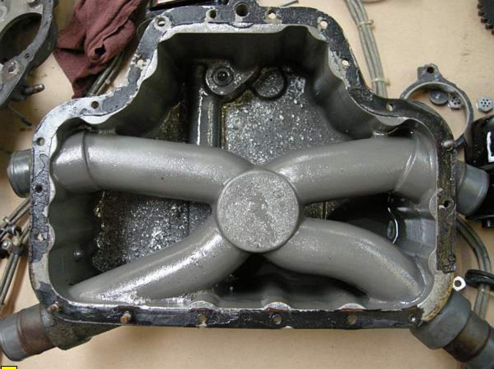
Photo 7 - Aluminum Shavings in bottom of oil pan
