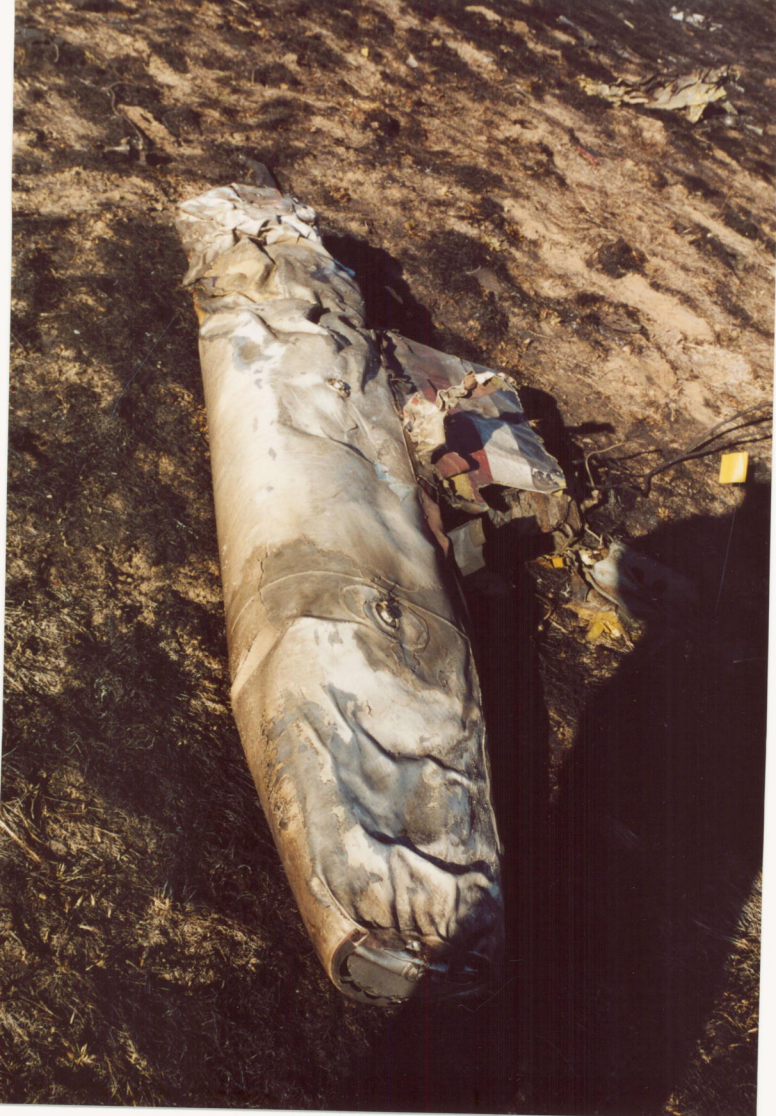
Photo 7 - A wing tip fuel tank (auxiliary tank).
