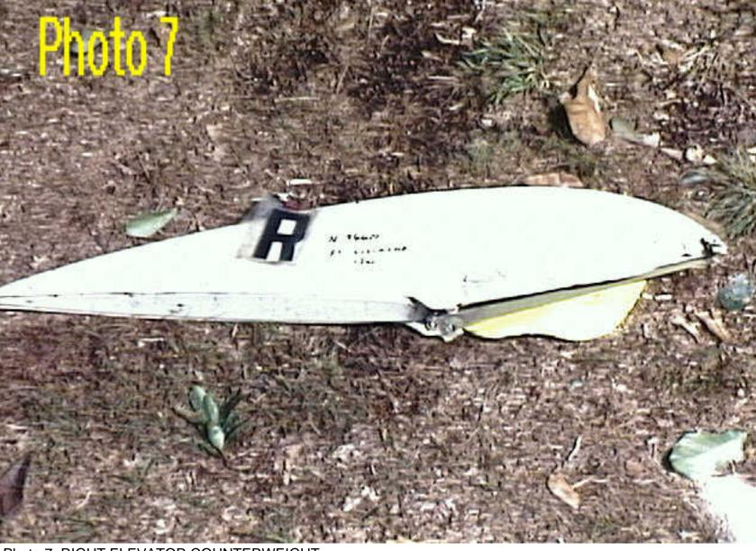
Photo 7: RIGHT ELEVATOR COUNTERWEIGHT.
