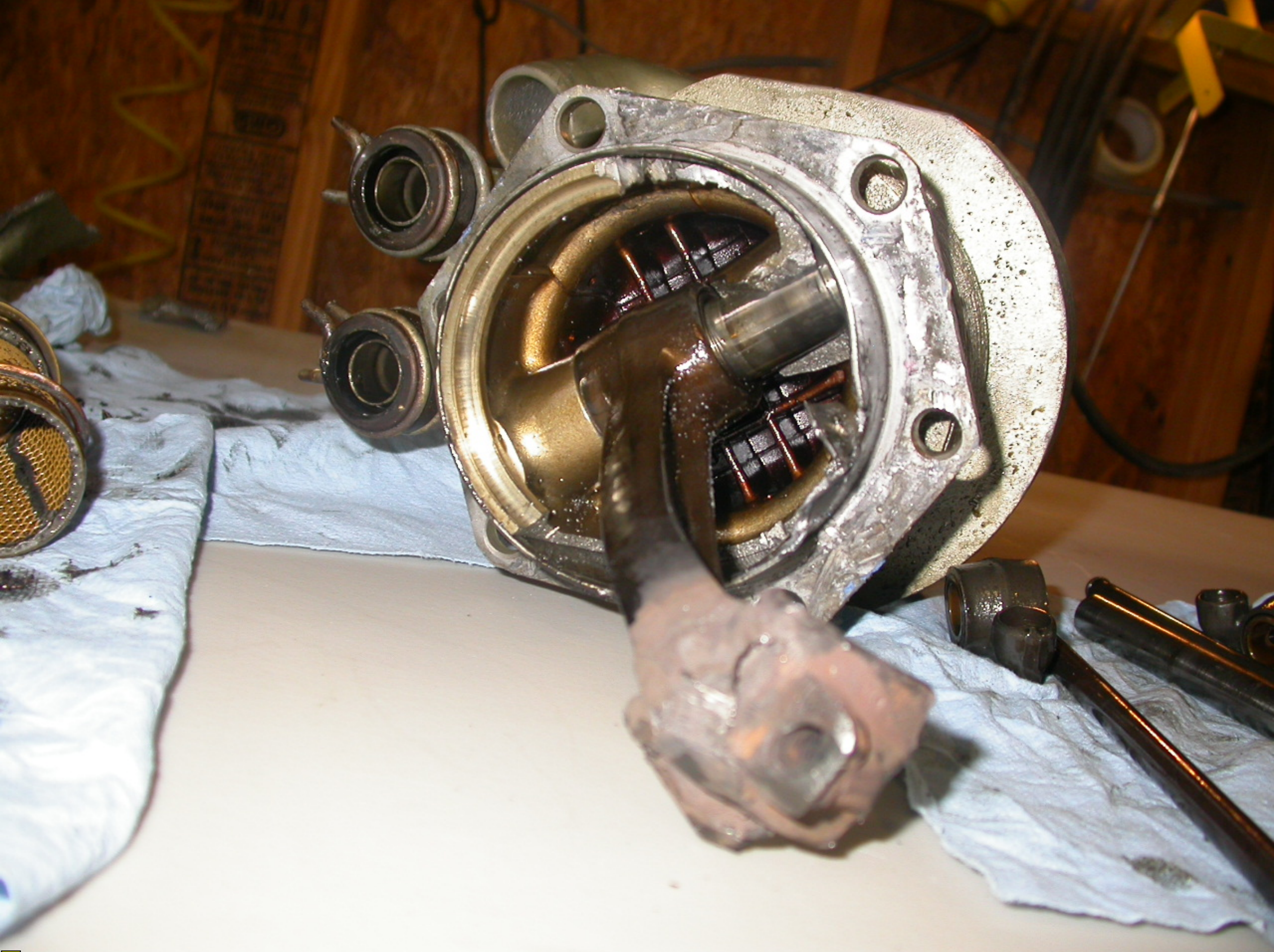
Photo 7: Number 2 piston rod damage.
