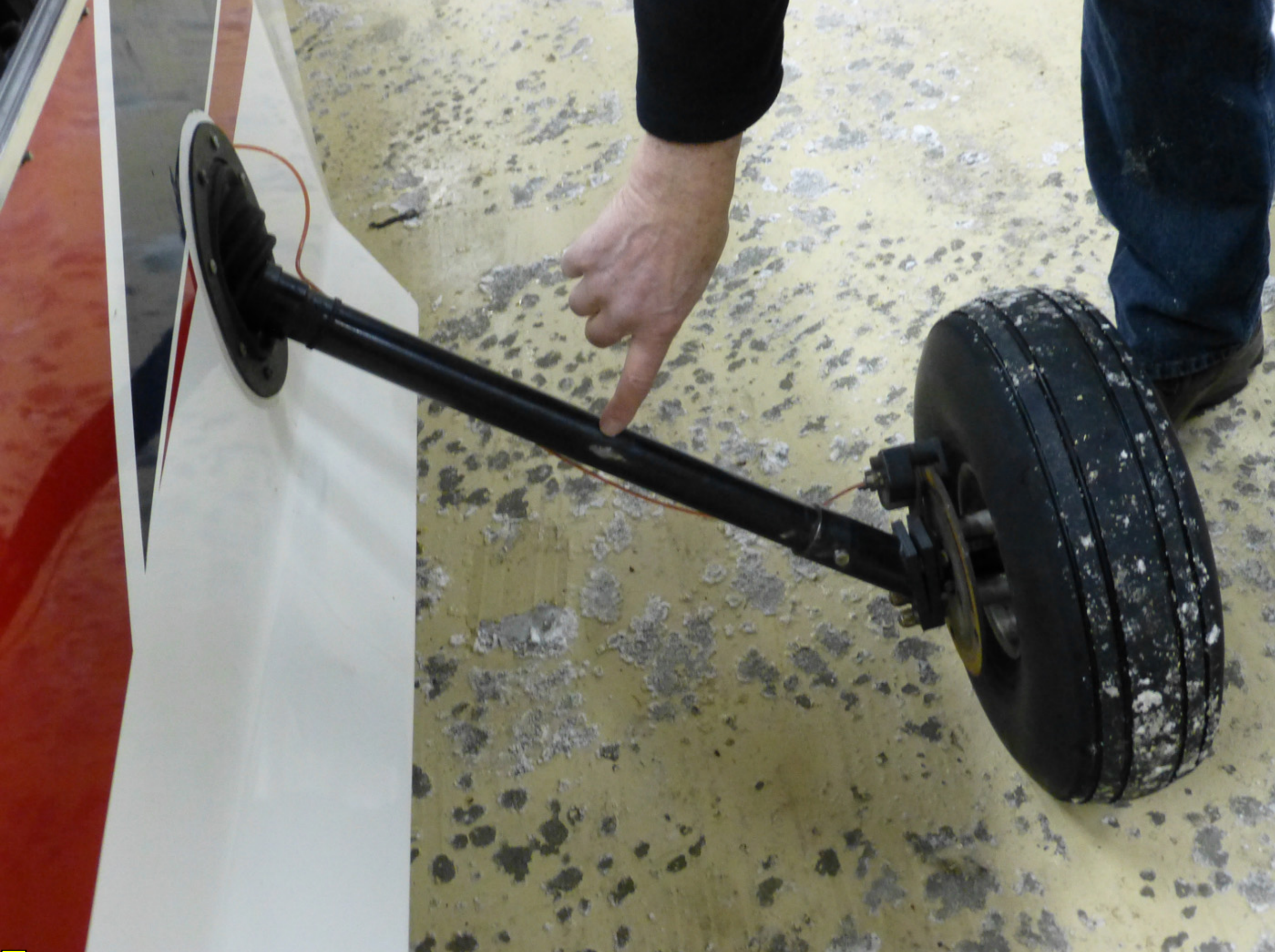
Photo 6. Wire Strike Mark, Left Main Landing Gear
