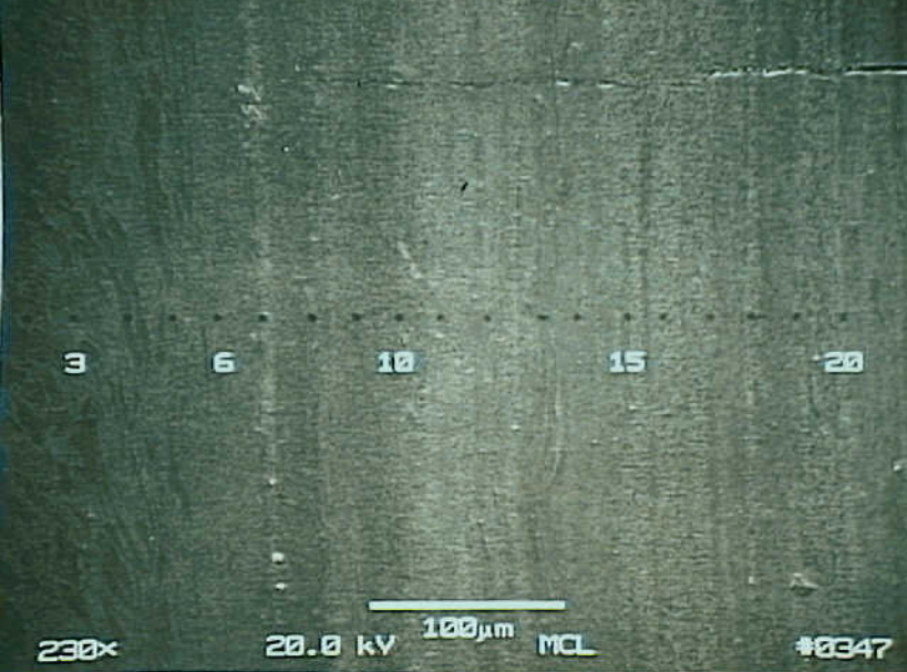
Photo 6. Cross section of hole #2B quite close to the location of the drill breakdown showing a surface layer with a appearance similar to the failed JT8-hub.
