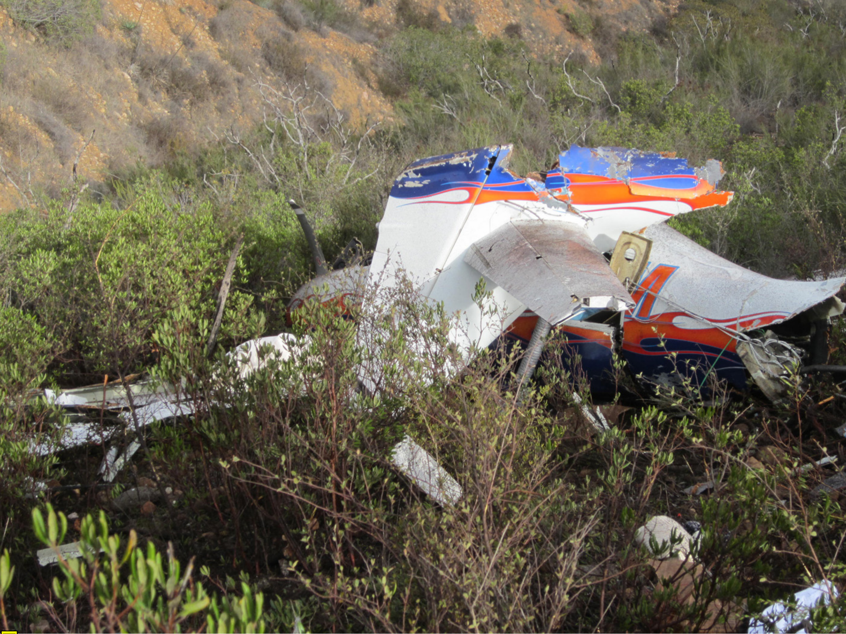
Photo 6 - Empennage broken off
