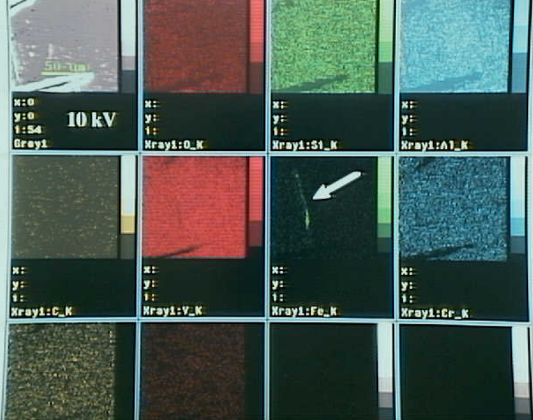
Photo 5. EDS map of the location labeled "A" in Region 1, Figure 4. An elevated concentration of K-bank iron was found in the patch of high intensity backscatter electrons (arrow).
