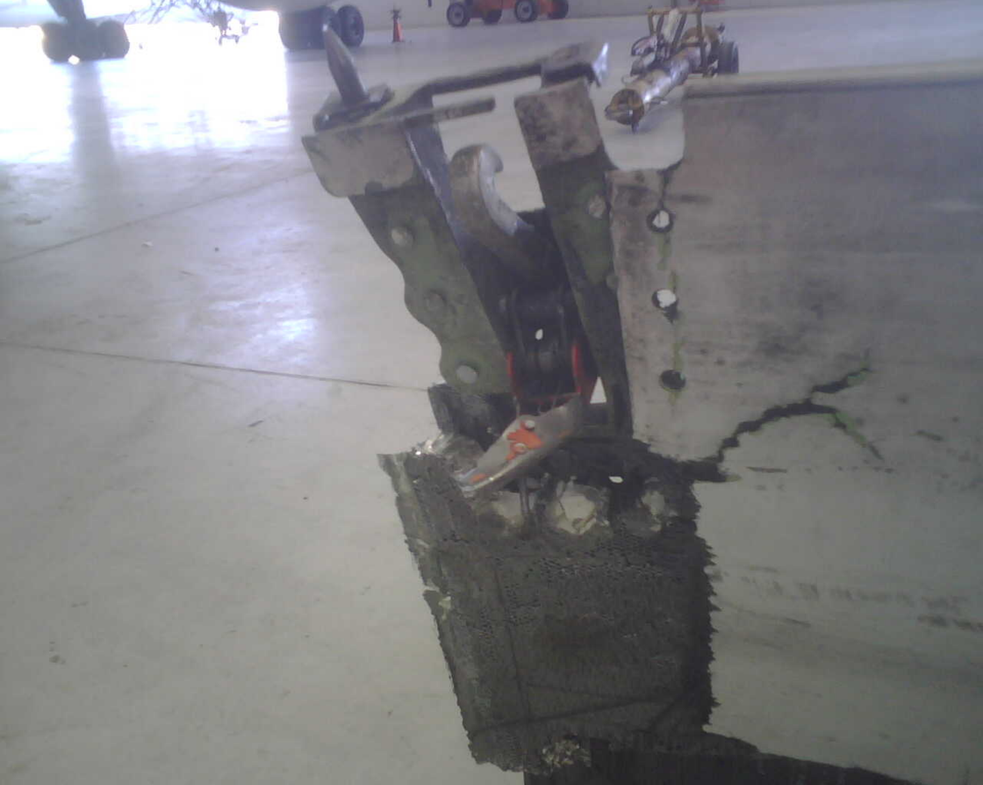
Photo 5. Damage to Engine Pylon Structure (FAA Photo)
