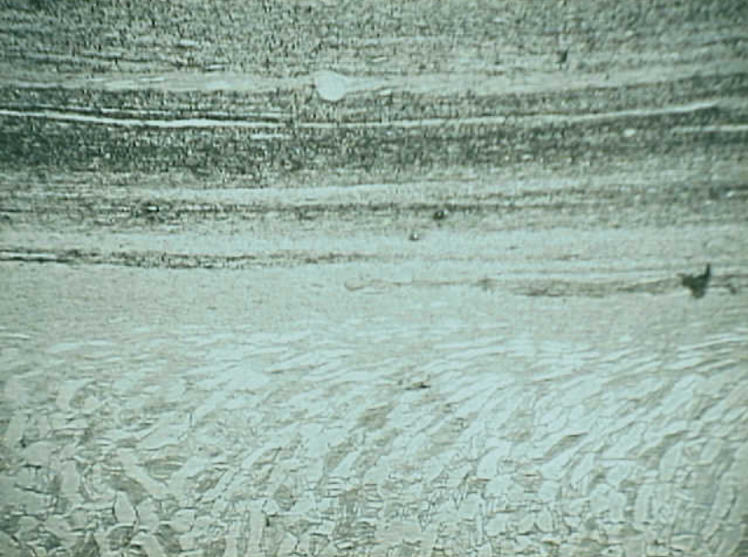
Photo 5. Cross section of hole #2B quite close to the location of the drill breakdown showing a surface layer with an appearance similar to the failed JT8-hub. Mag. 128X.
