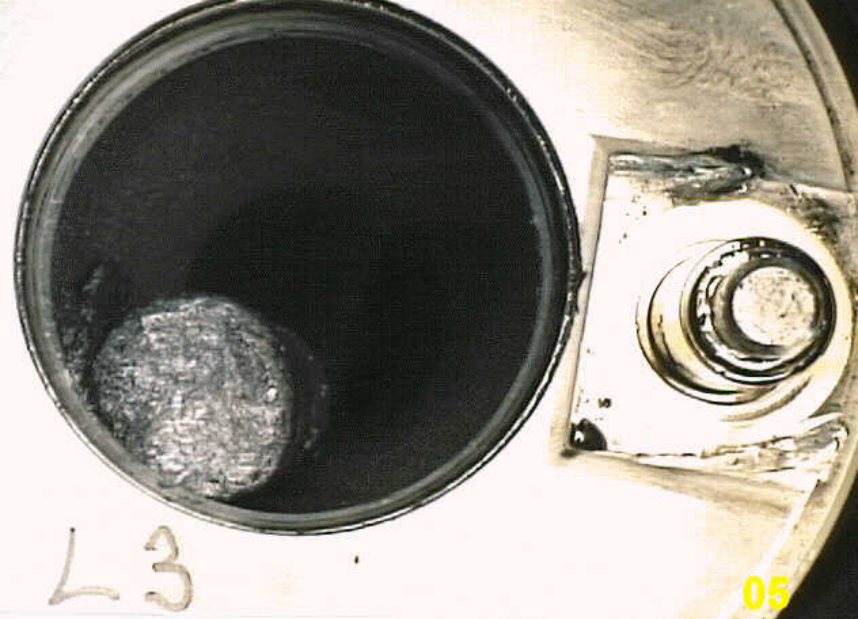
Photo 5 Left Engine and Propeller-No.3 propeller blade taper bore and pitch change pin
