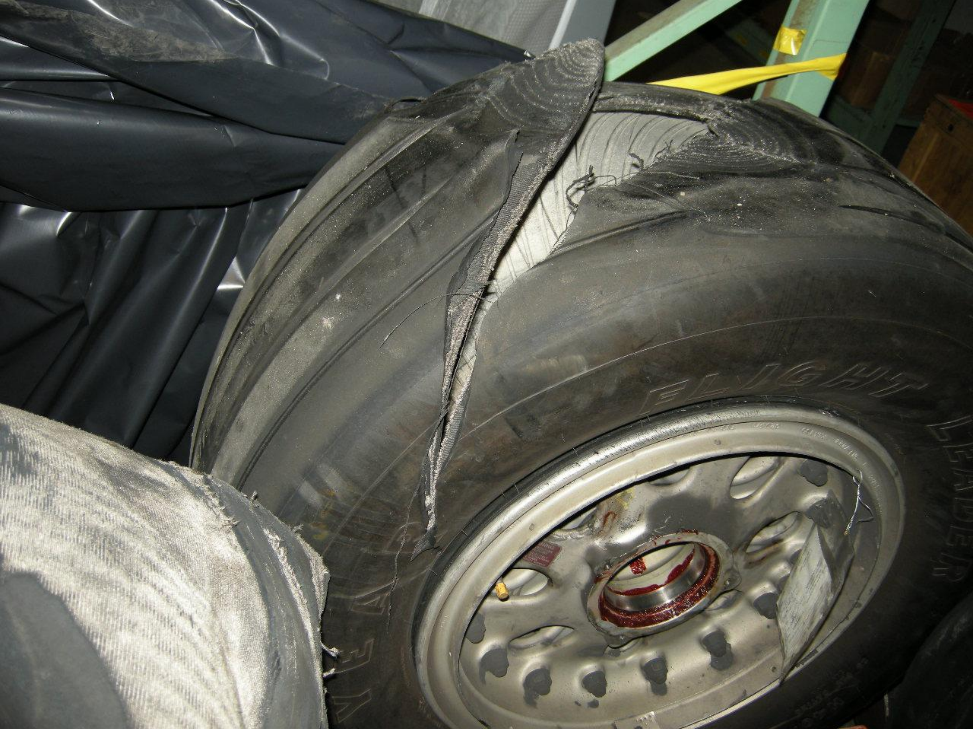
Photo 5 - Showing Damage to Left Outboard Tire
