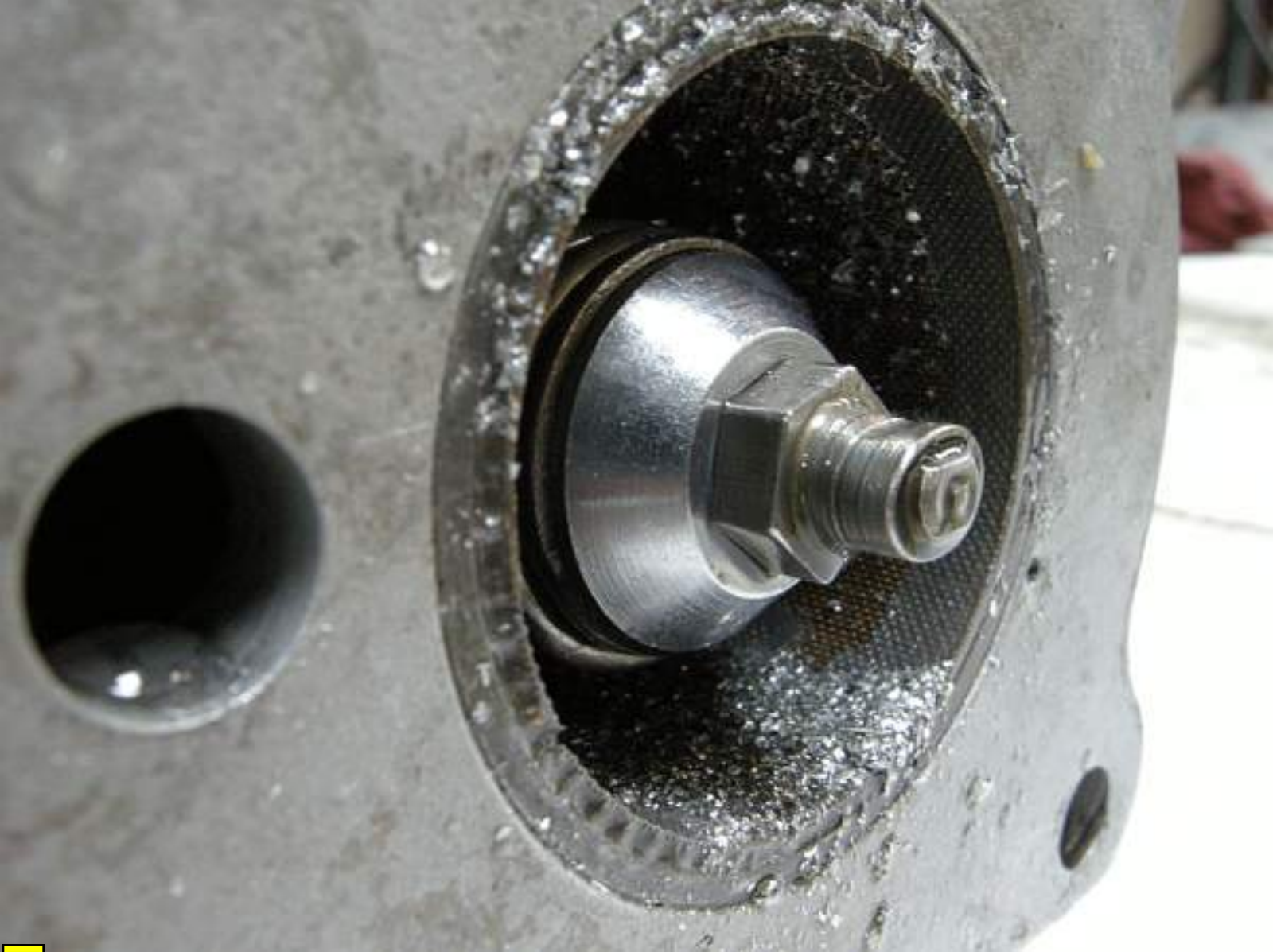
Photo 5 - Metal Shavings in the Vernatherm and Housing
