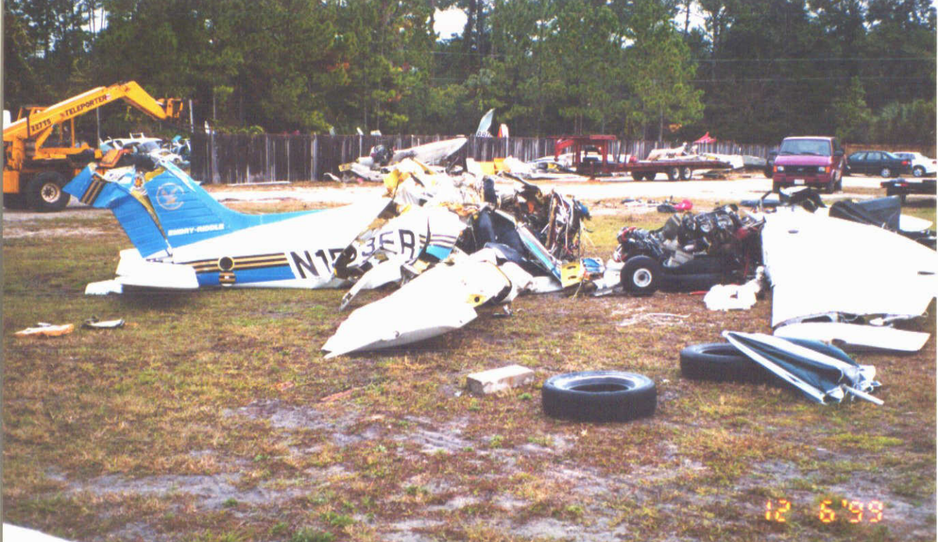
Photo 5: View of the Cadet with a section of the left wing and left engine from the Seminole visible.
