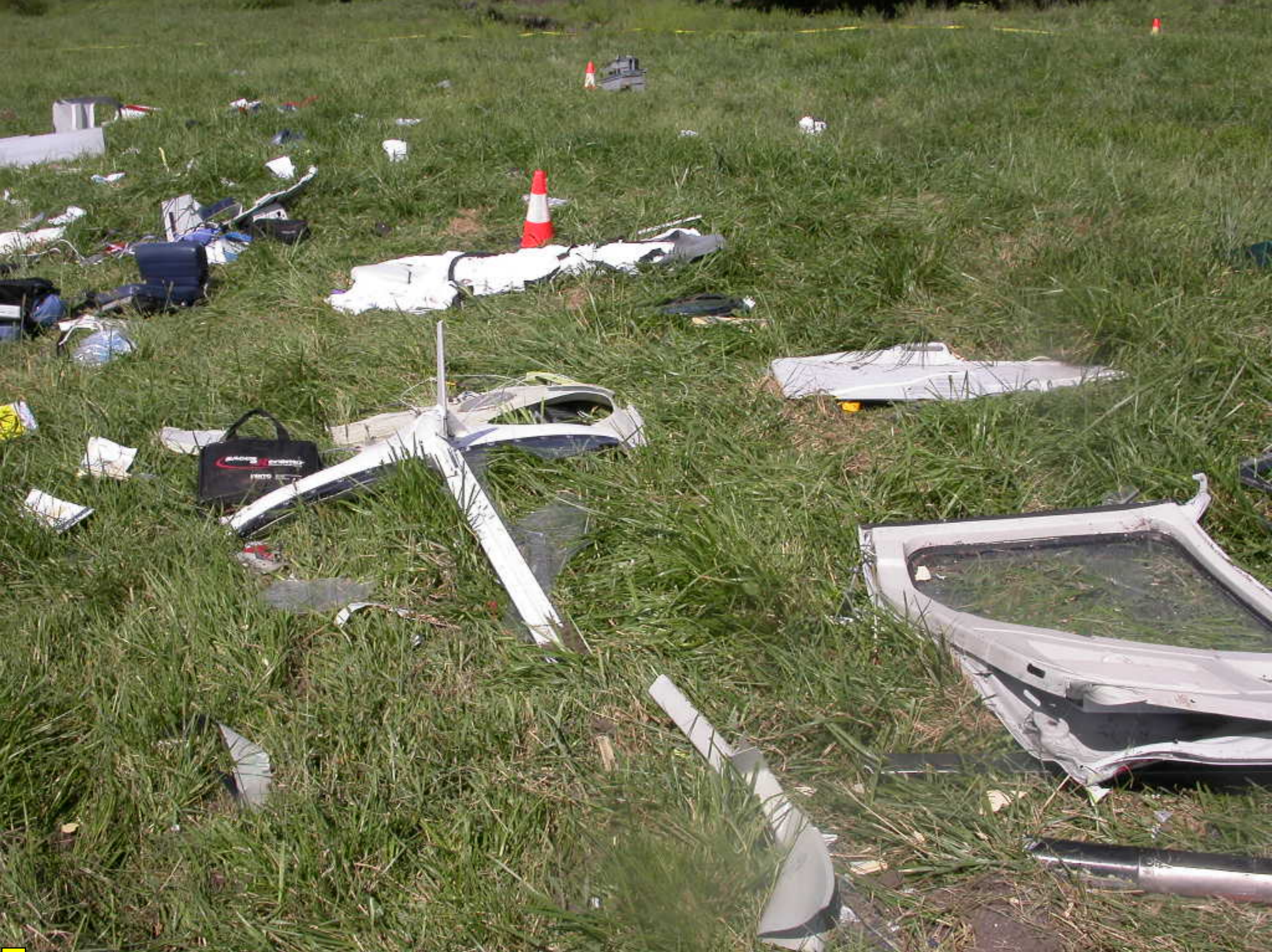
Photo 5: Debris field with view of wire cutter and windshield frame
