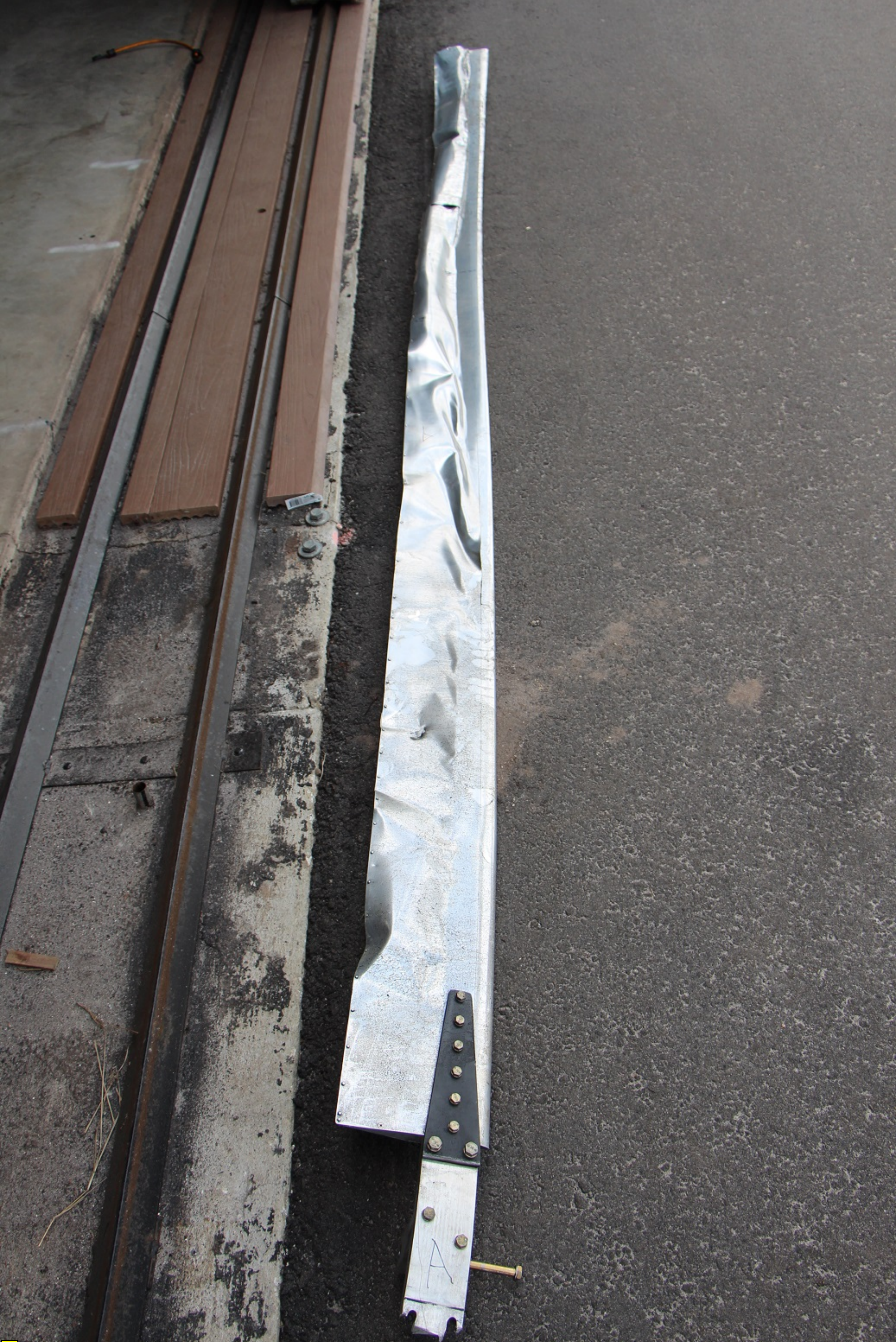
Photo 1: Blade A Damage.
