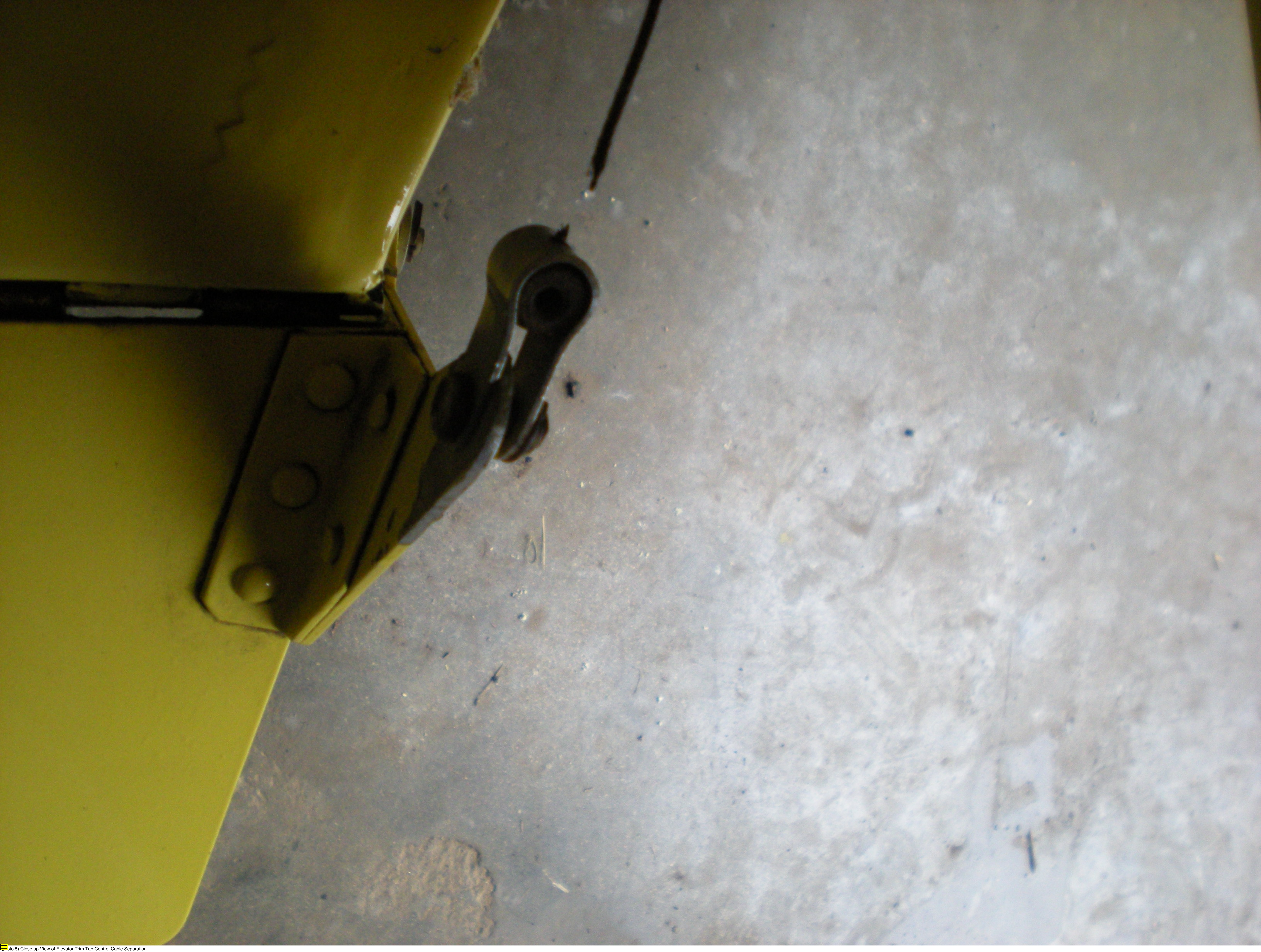
Photo 5) Close up View of Elevator Trim Tab Control Cable Separation.
