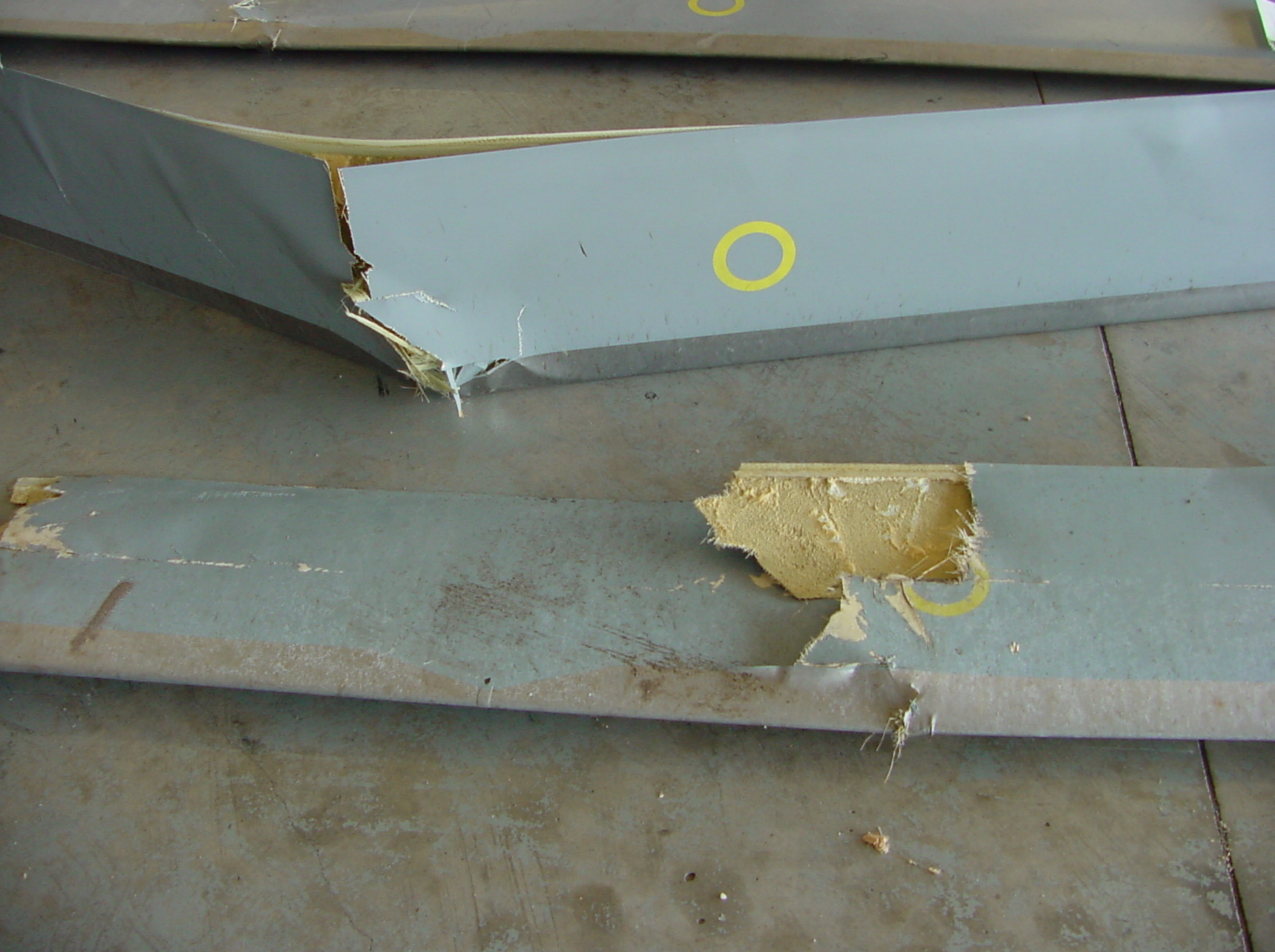
Photo 44. Inboard Fracture on Blue Main Rotor Blade. Yellow Main Rotor Blade in Background (Eurocopter Photo)
