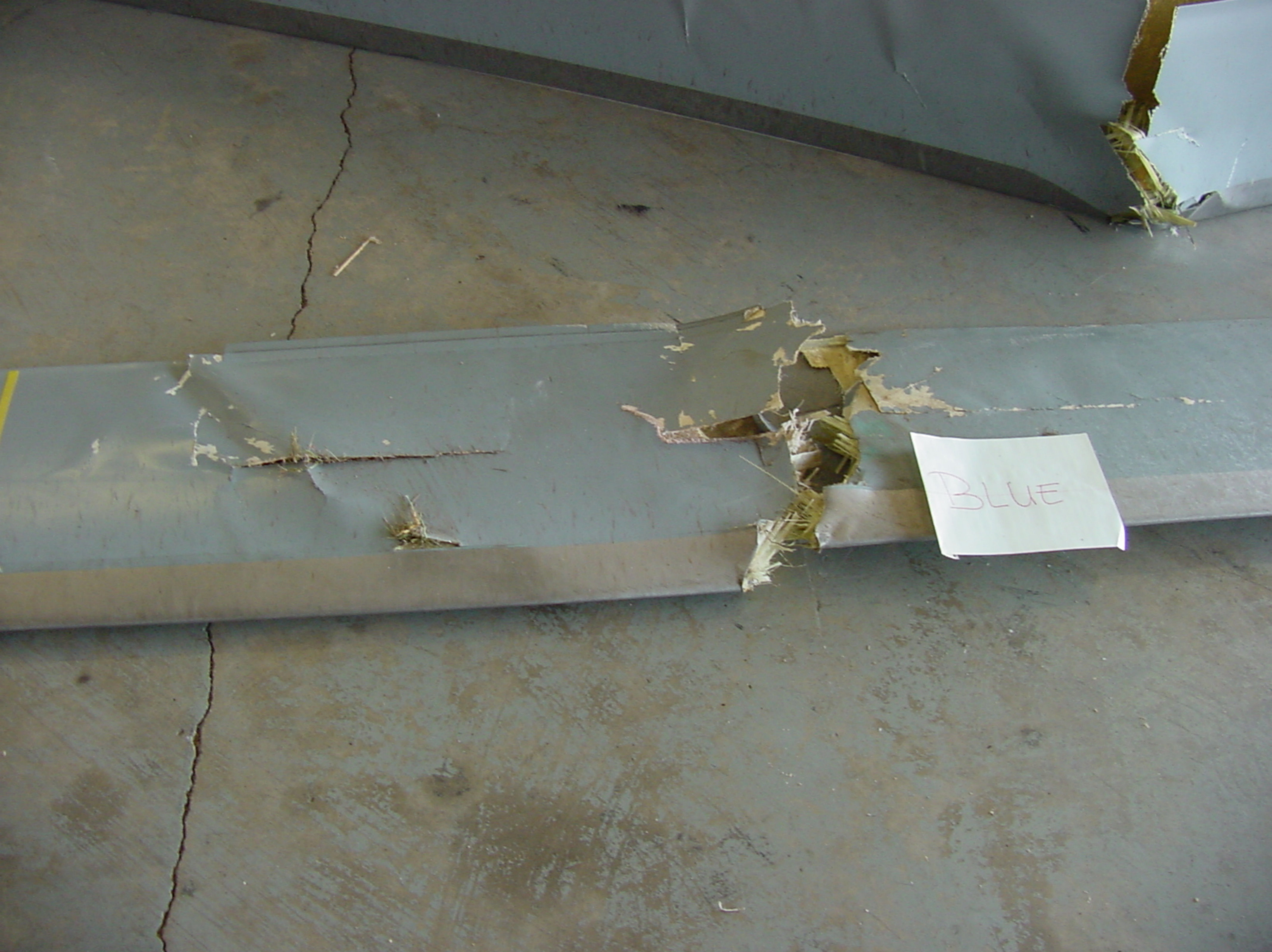
Photo 43. Outboard Fracture on Blue Main Rotor Blade (Eurocopter Photo)
