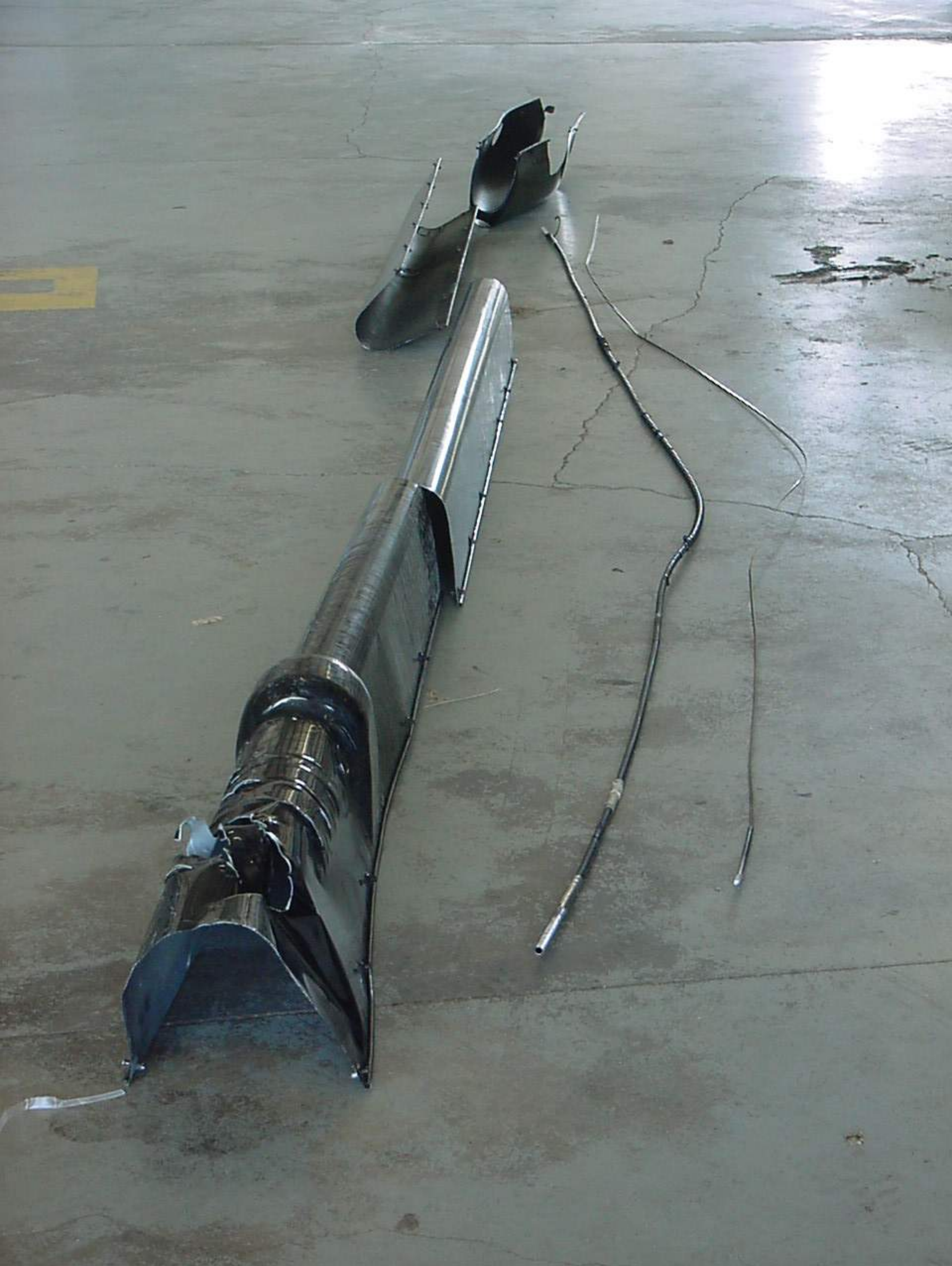
Photo 40. Tail Rotor Drive Shaft Cowling and Control Cable
