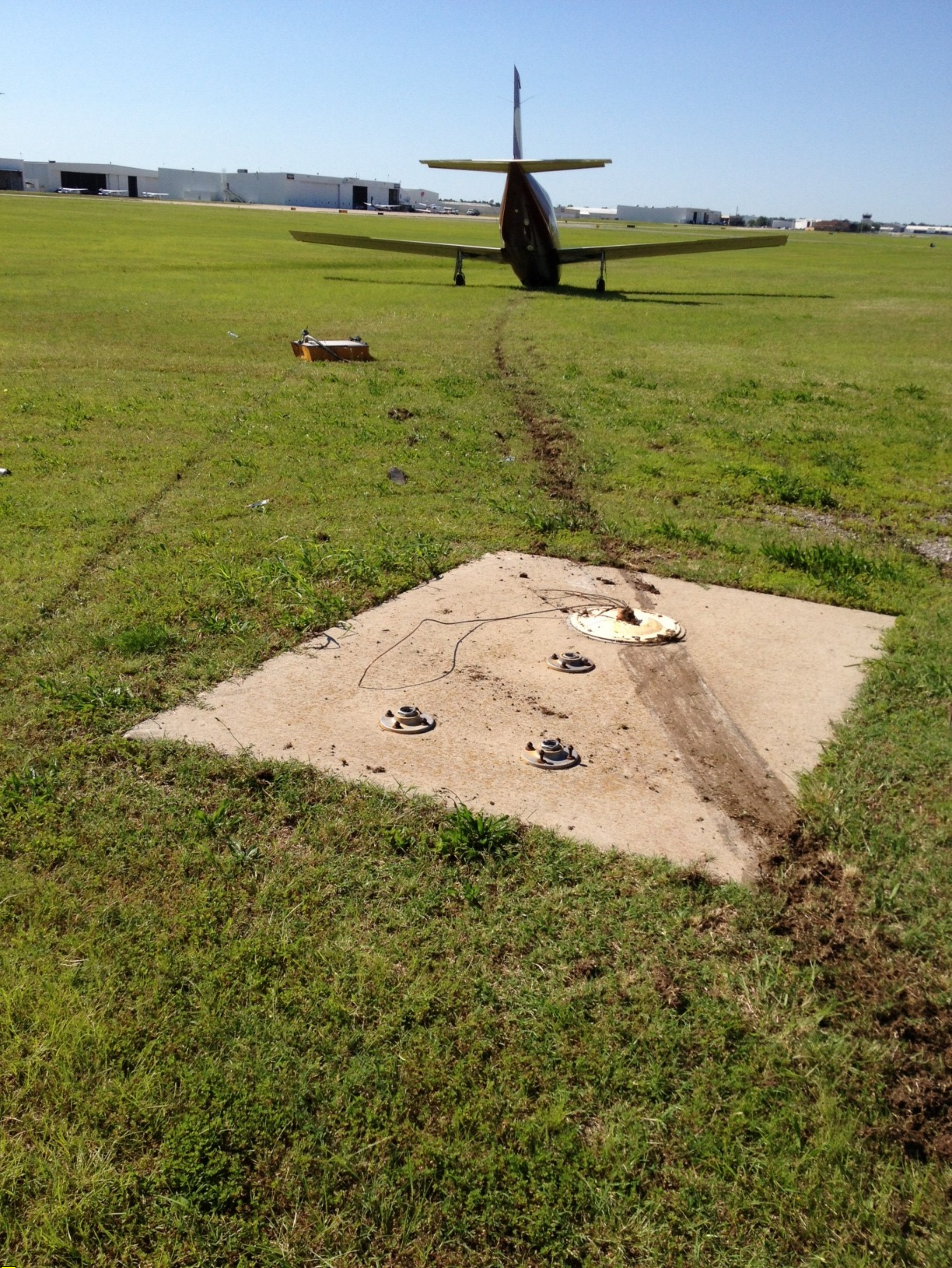
Photo 4. View of the PAPI light struck by the airplane.
