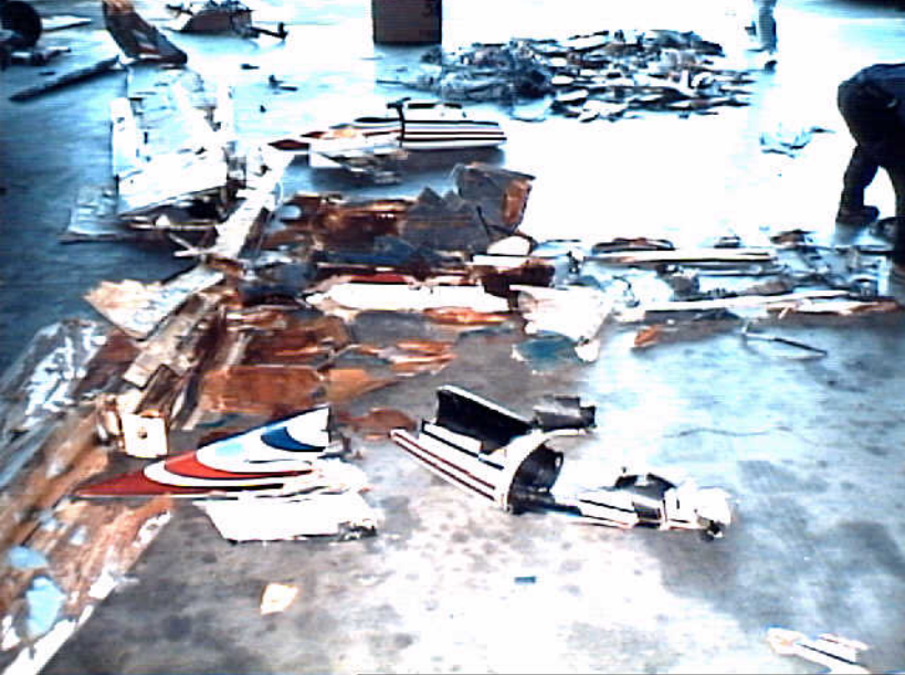
Photo 4. Wreckage layout of center section and cargo pods.
