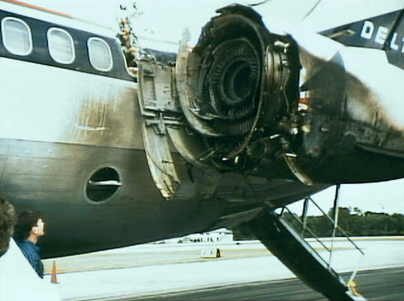
Photo 4. Left fuselage and engine damage, including fire damage to nacelle.
