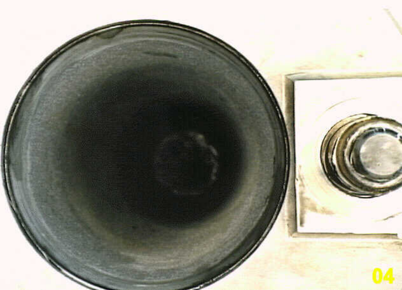
Photo 4 Left Engine and Propeller-No.1 propeller blade taper bore and pitch change pin
