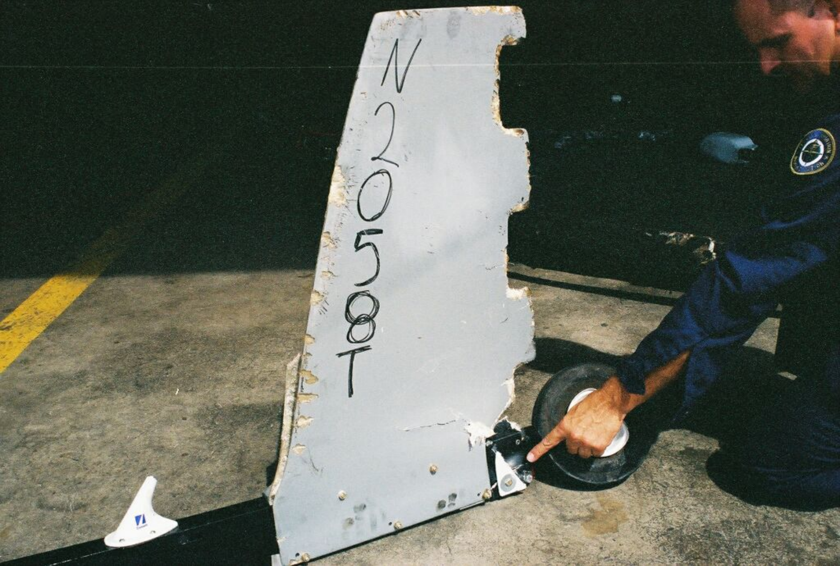
Photo 4 - Vertical stabilizer. Note chop marks on leading edge.
