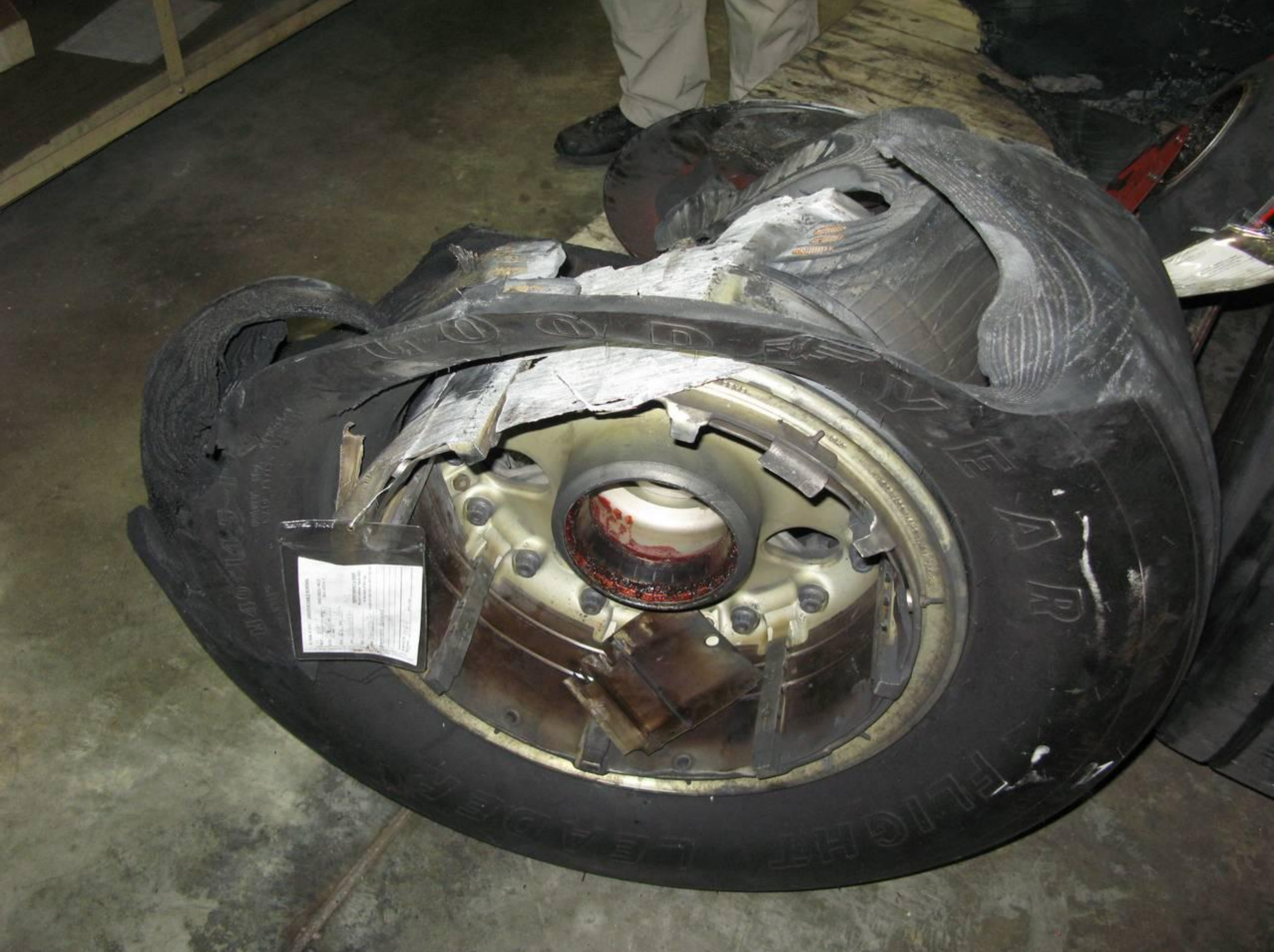
Photo 4 - Showing Damage to Right Outboard Tire
