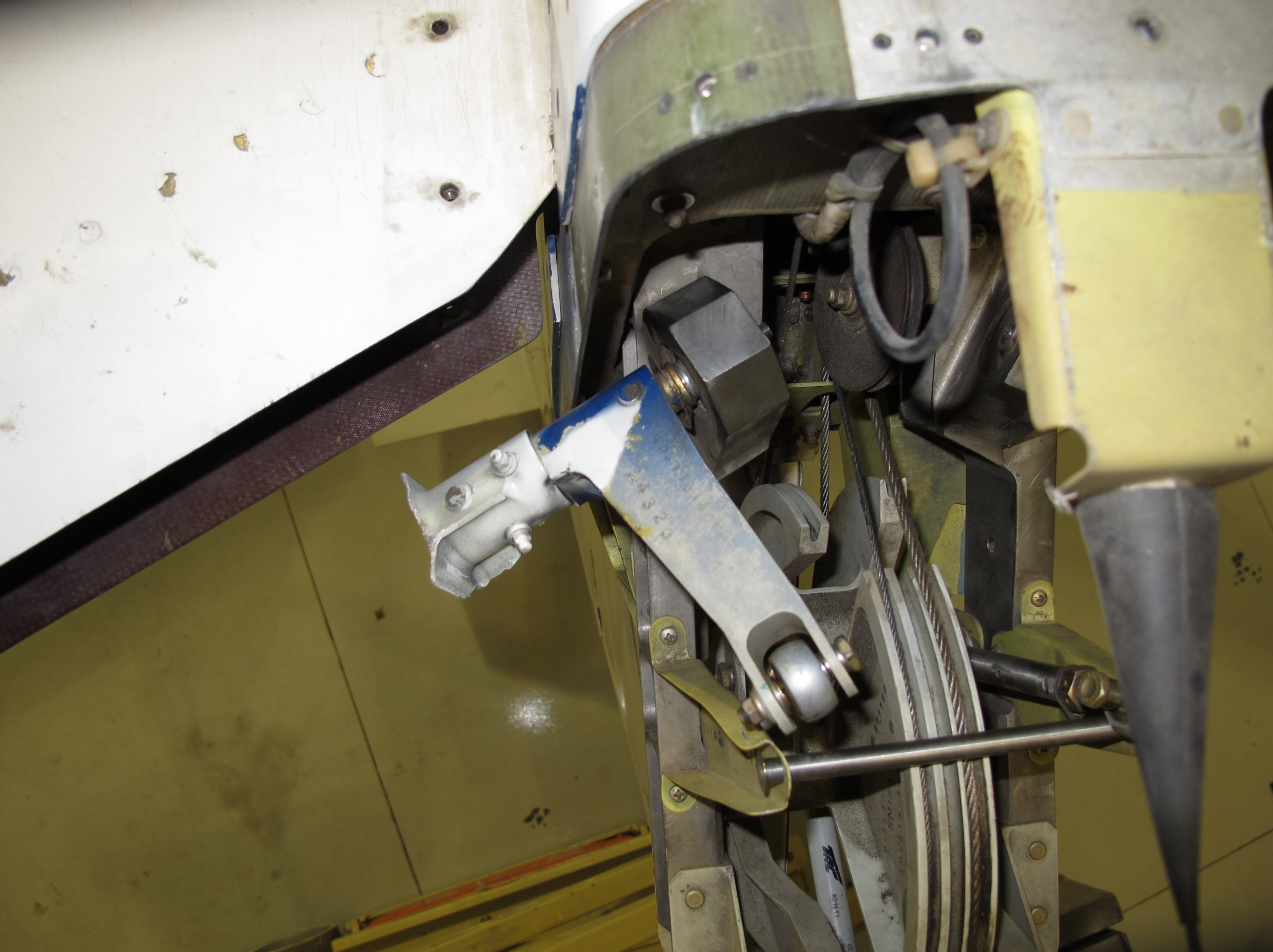
to 4 - Left elevator bell crank
