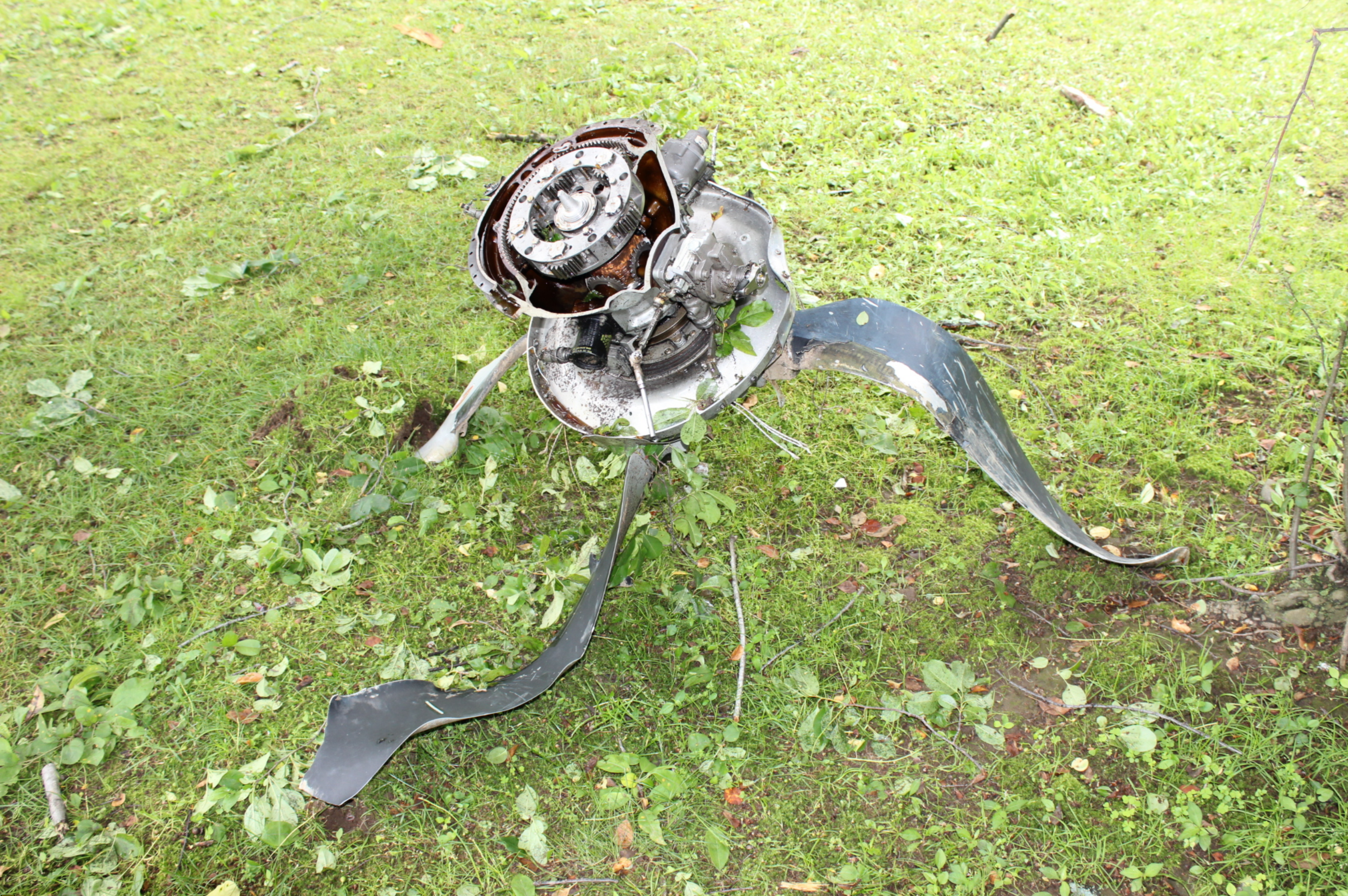
Photo 4 - View of Propeller and Gearbox Assemblies (PWC)
