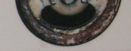
LEAD FOULED Hard, cinderlike deposits from poor fuel vaporization, high T.E.L. content in fuel or engine operating too cold. Install new Champions.
