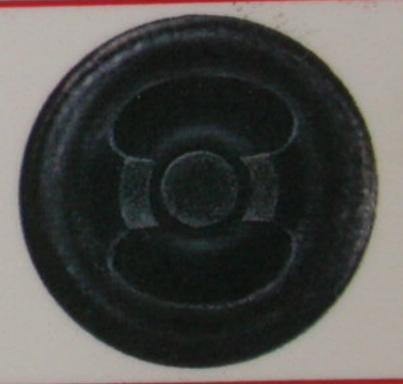
OIL FOULED Wet, oily deposits may be caused by broken or worn piston rings, excessive valve guide clearances, leaking impeller seal or engine still in break-in period.
