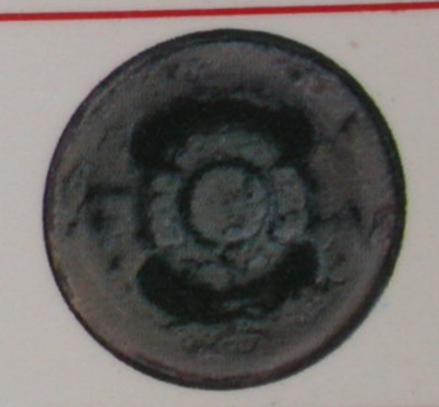
CARBON FOULED Black, sooty deposits from excessive ground idling, idle mixture too rich or plug type too cold. If heat range is correct, clean, regap, test and reinstall.
