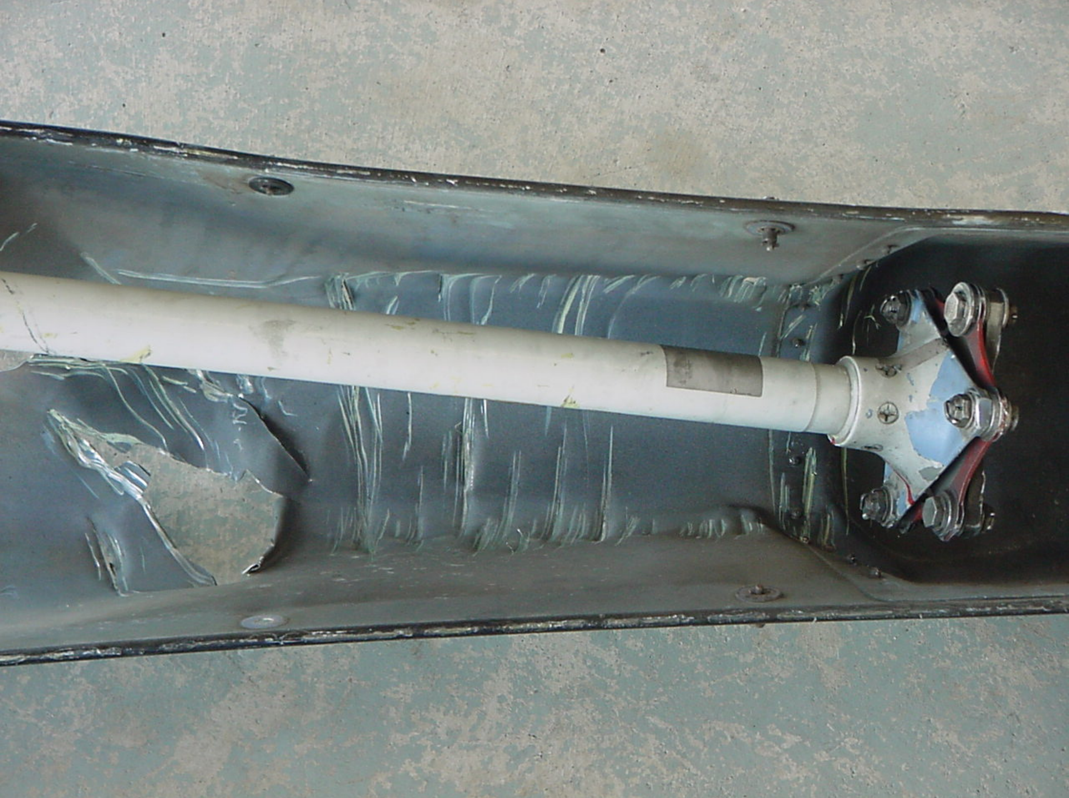
Photo 39. Cowling Which Houses the Tail Rotor Drive Short Shaft
