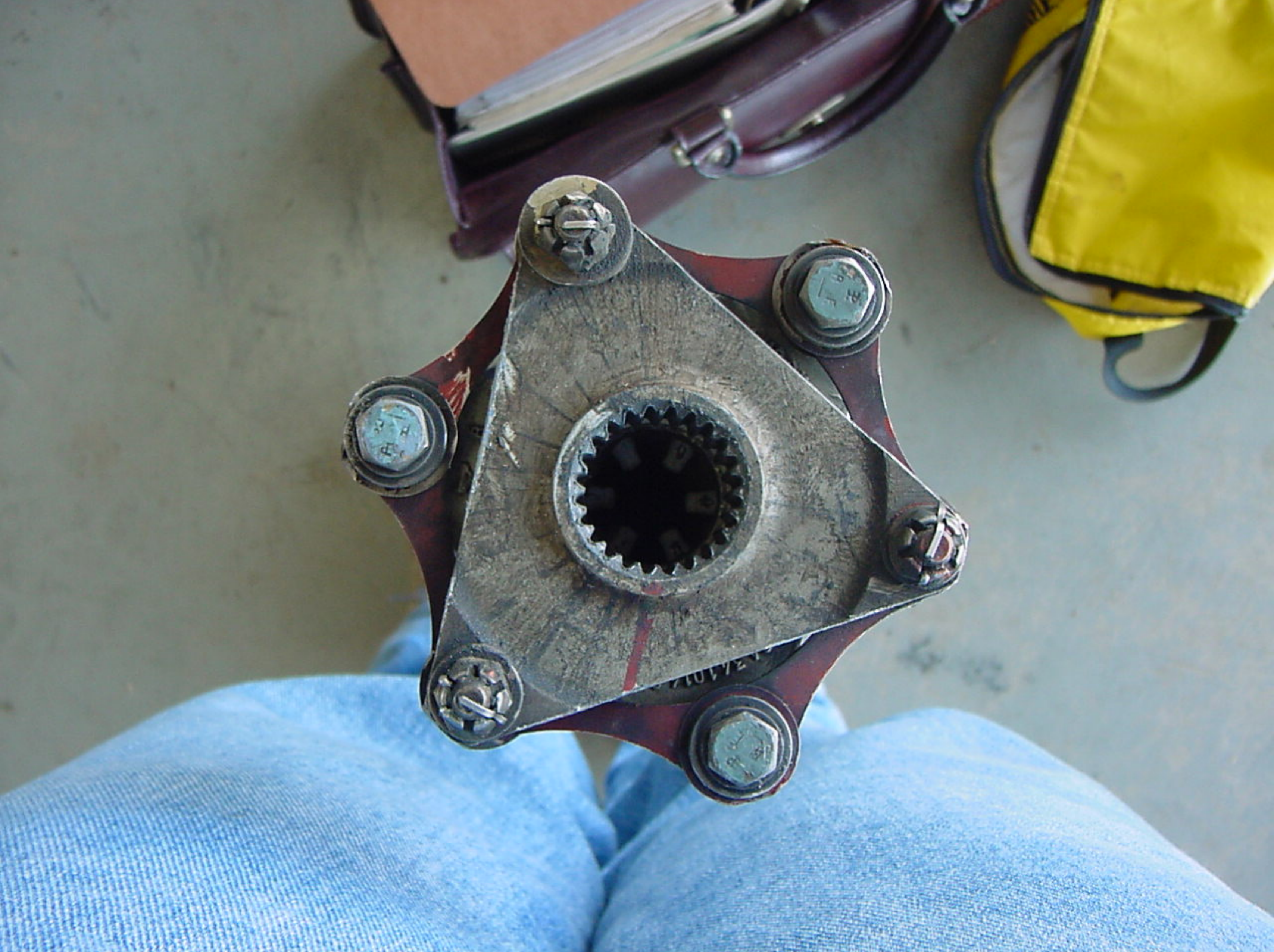
Photo 38. Rear Coupling on the Tail Rotor Drive Short Shaft
