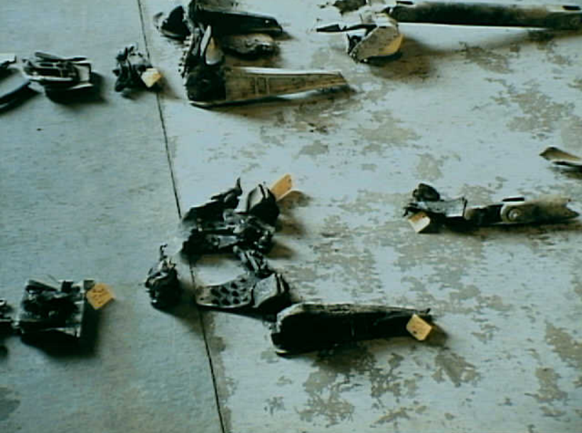
Photo 38. No. 1 & 2 engine and pylon mounts and thrust links
