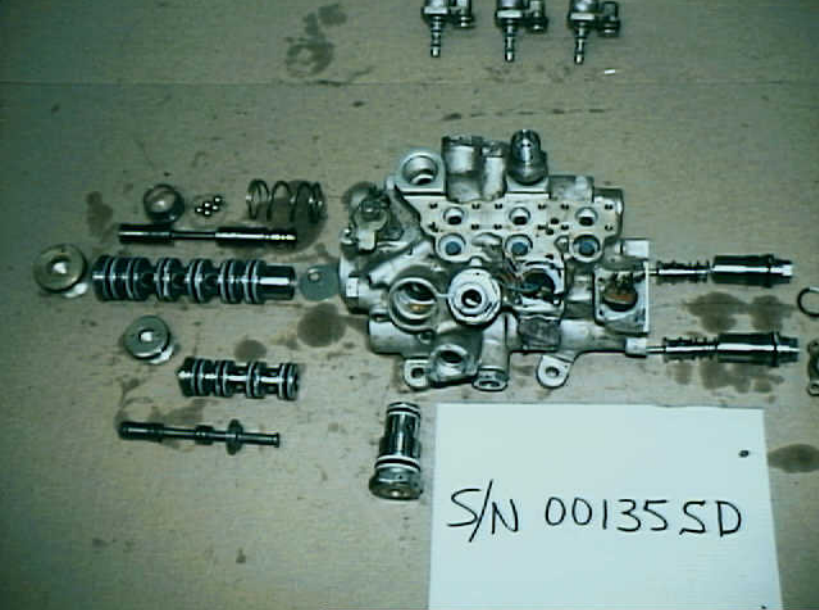
Photo 35. No. 2 engine reverser control valve module
