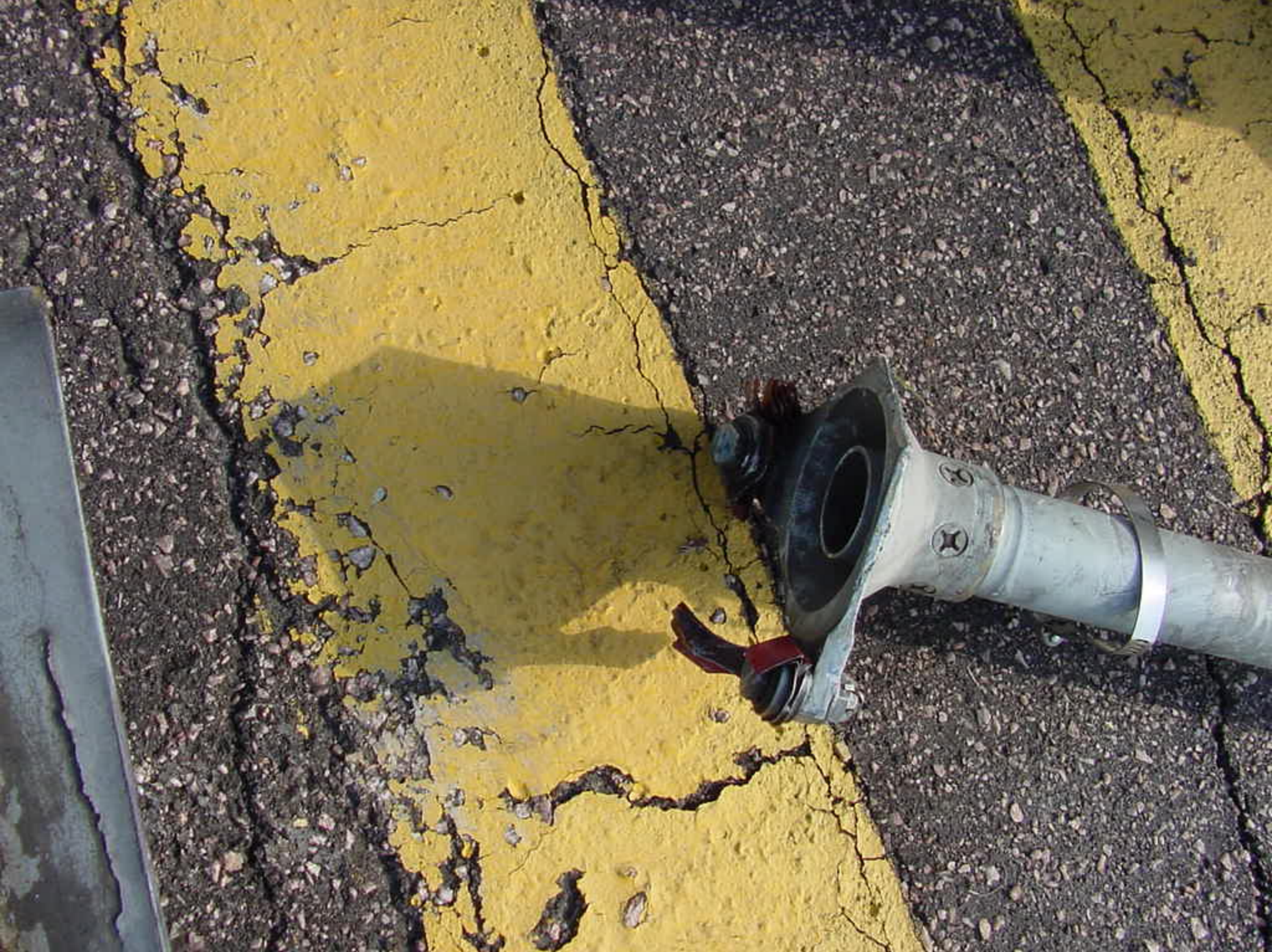
Photo 34. Forward Coupling on the Tail Rotor Drive Short Shaft (Norfolk Police Photo)
