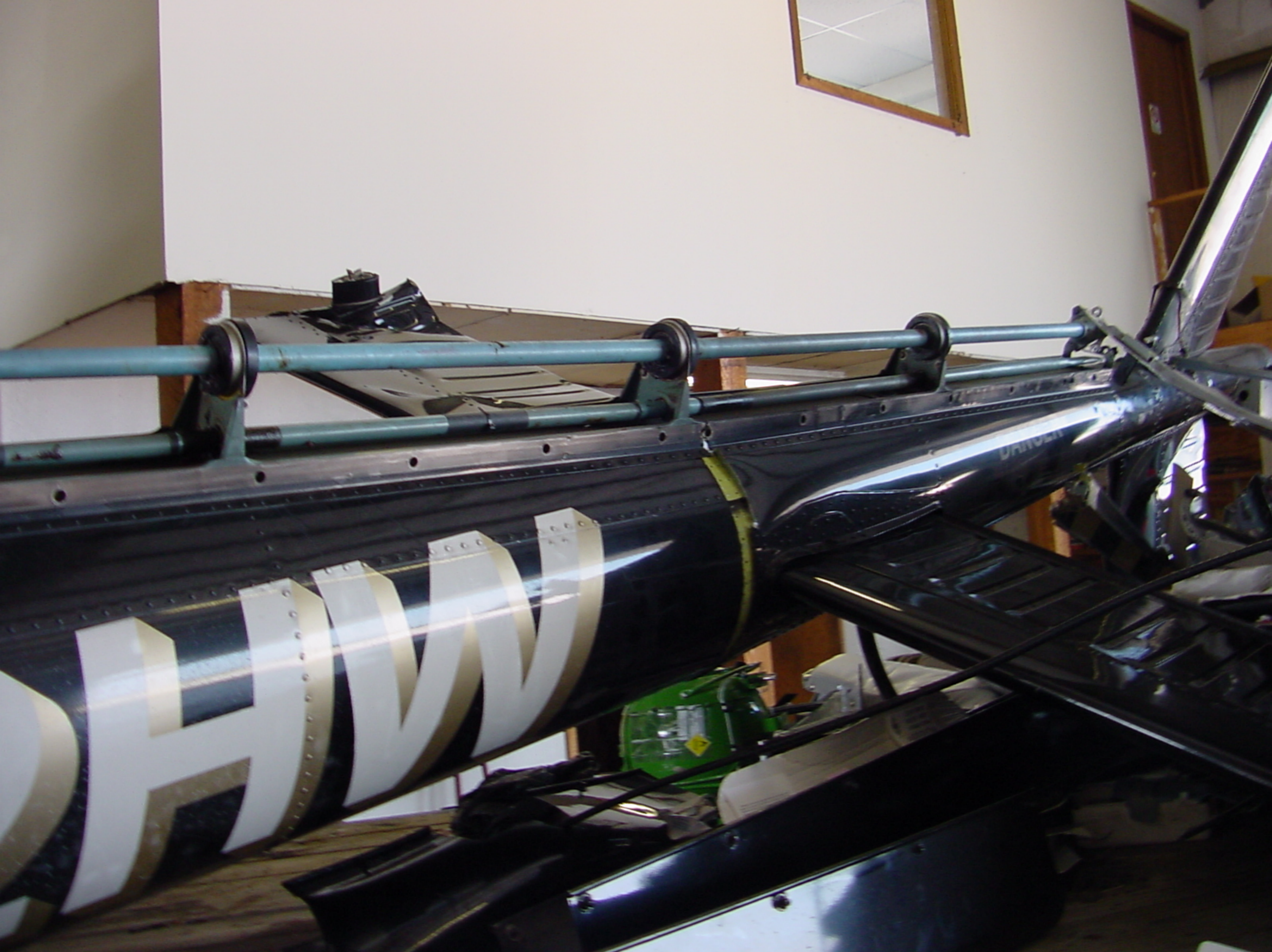
Photo 33. View of Other Brackets Along Pitch Change Rod (Eurocopter Photo)
